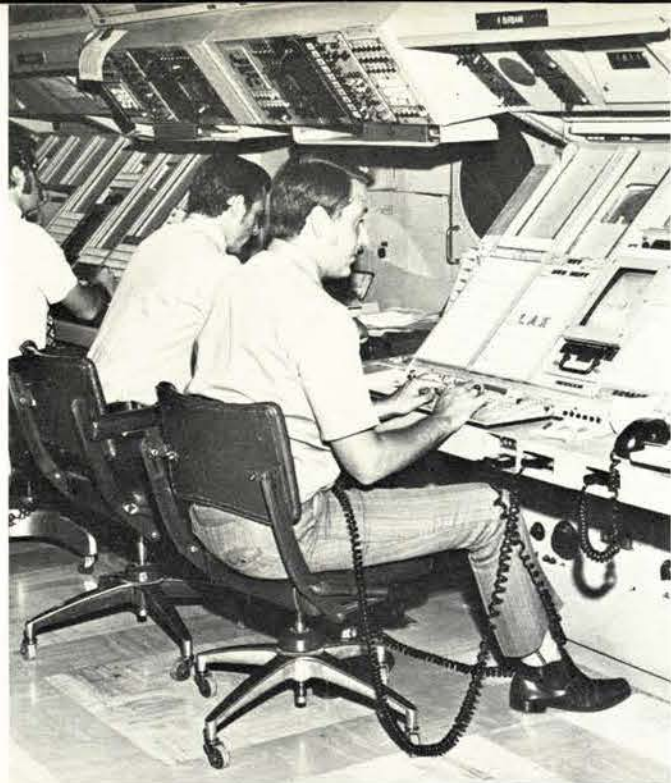
State-of-the-art in en route center equipment at Los Angeles involves radar and computer update equipment (CUE) for entering the flight-plan data. At the computer entry device (CED) is an alphanumeric computer readout.
