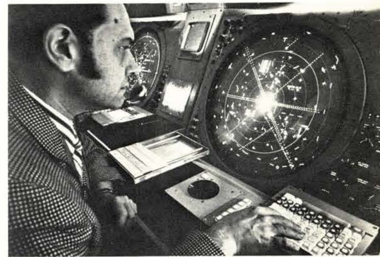
The first field facility to get the Automated Radar Terminal System was Chicago O'Hare. The controller watches a display that automatically shows the identity, altitude, speed, range and bearing of aircraft in the terminal area.
