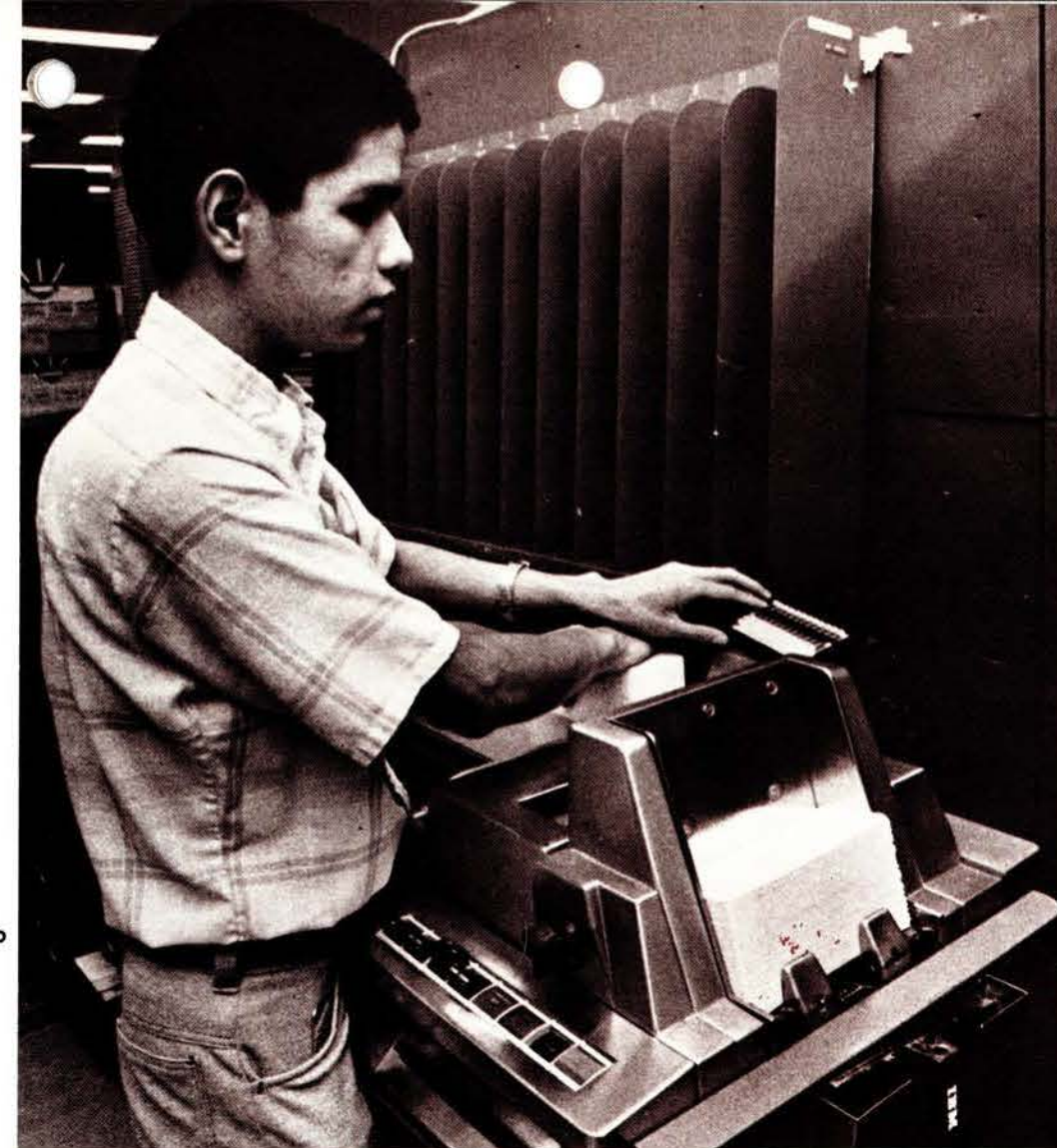
Chong uses an abacus held in place by magnets to keep track of the card columns being sorted and the number of cards he has processed during a run.
