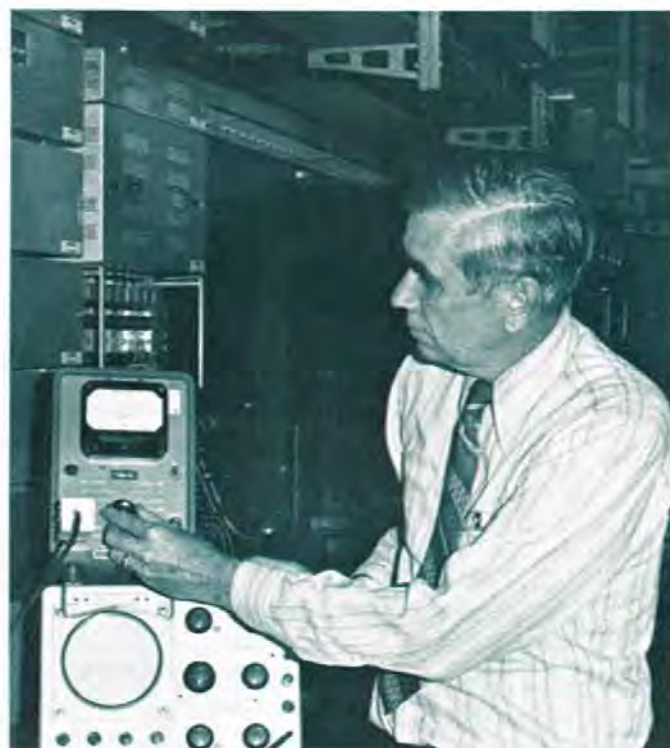
Technician Gene Stevens gets the voltmeter and oscilloscope ready before starting the diagnosis for a maintenance job he's doing on the microwave-link terminal
