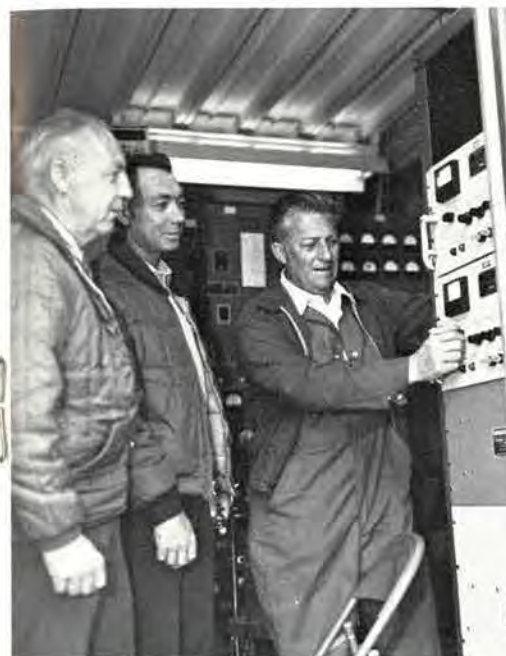
NEITHER SLEET NOR —Denver Sector personnel worked through unseasonable snow and heavy rain to convert the Runway 35 glide slope to the "capture effect." Engineer George Beasley (right) checks new solid-state ILS clearance transmitter with Nav aids chief Harry Mogensen (left) and electronic technician Fred Weaver.
