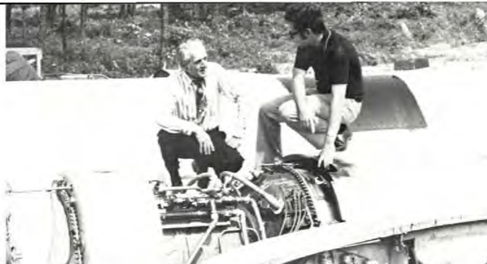
Engineers Julius Gassmann (left) and Richard Hill are working on devices to detect fuel-leak fires that burn holes in engine burner cans.
