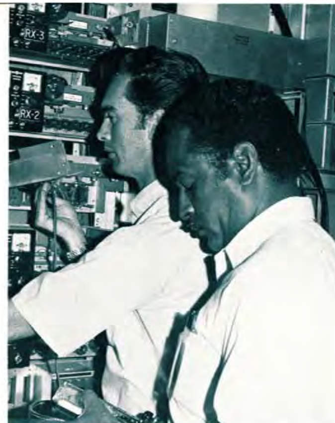
Repairing a microwave-link terminal at the Washington En Route Center are technicians Doug Huskins (left) and George Brown, who is keeping his eyes on a voltmeter.
