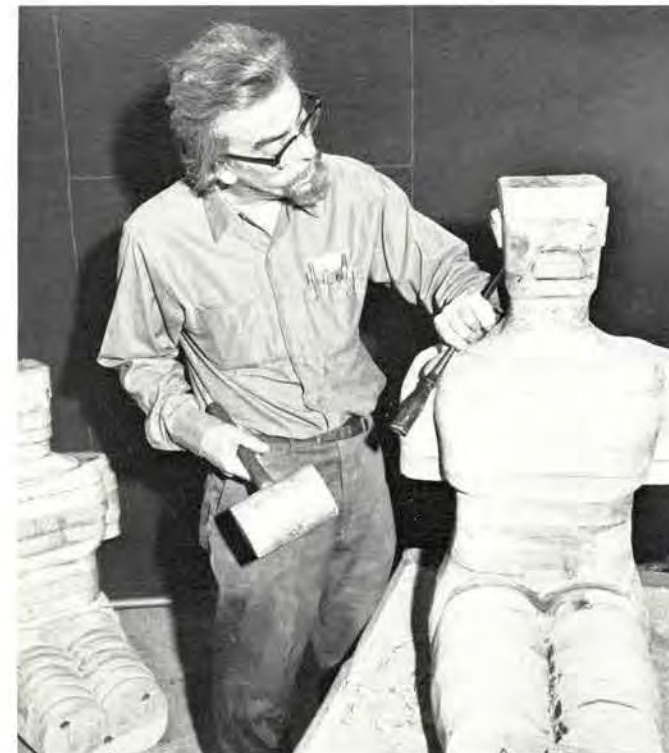
MAKER OF MEN —Modelmaker Edwin J. Call chisels away at a wooden dummy to be used in airplane seat tests at NAFEC. The needed rigid dummies cannot be bought, so Call had to design, build and sculpture them.
