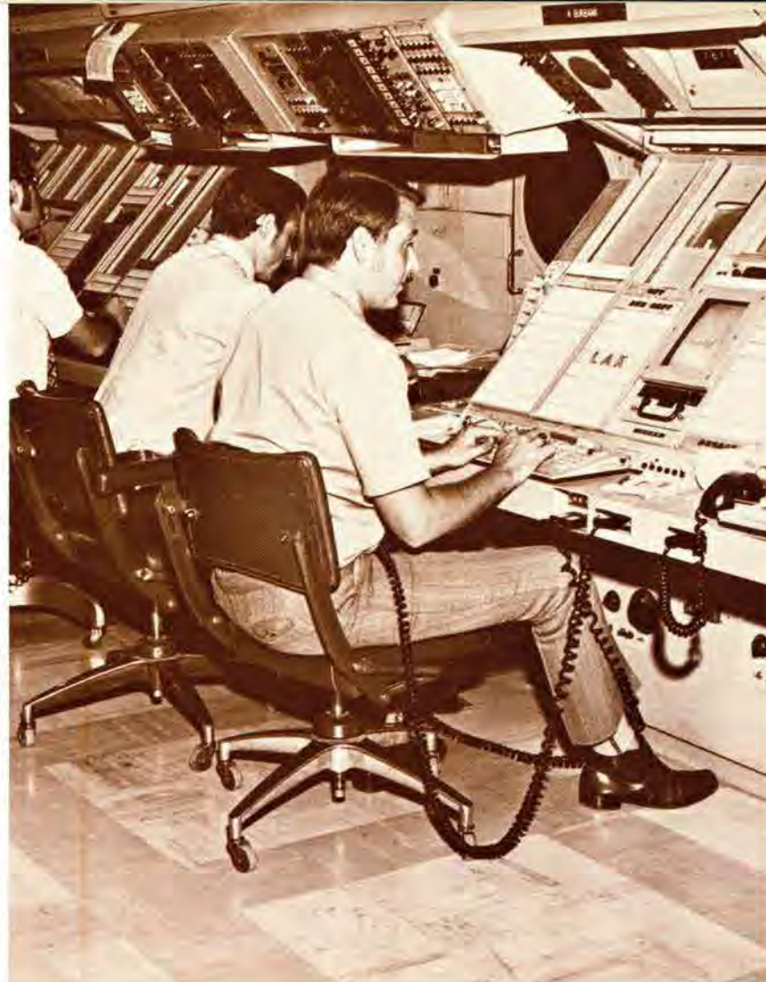
ATCS Alan Adgate mans the radar position as ATCS Mike McDaniel enters flight-plan data via a computer entry device (CED), part of the computer update equipment at Los Angeles. The square screen in front of him is an alphanumeric computer readout, and the six-button panel to the keyboard's right is a Quick Action Keypack (QAK), which permits McDaniel to enter some information quickly.
