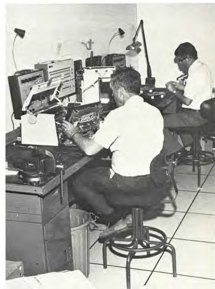
Repairing a computer IOT and a computer update equipment (CUE) keypack are Los Angeles center AF sector technicians Guy Manseill (left) and Roland DeMond.
