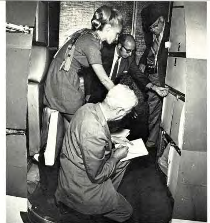
With jump seats in this position, many a stewardess plants her feet against not-too-secure galley storage lockers. Continental Airlines stewardess Hillary Thompson, an ALPA safety chairman, points to a bottom locker with basket too shallow to engage thumb latches when sliding out. Fred Jenkins of FAA's Los Angeles Systems and Equipment Branch tries out a thumb latch, which inadvertently could be left in the open position, as inspector Bernard Grochal takes notes and inspector Raymond Wells observes.
