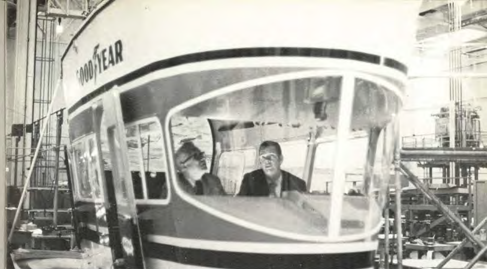
Reviewing installation of the control panel in the new "Europa" airship car, Inspector Dick Hansen (left) is accompanied by Goodyear Aerospace's Clarence Gibson, manager of quality assurance. The agency recently issued a production type certificate for Goodyear blimps, which heretofore were built and type certificated on an individual basis. Airlifted to and assembled in England, the fourth and newest blimp will be a goodwill ambassador over European sporting events in spring and summer.
