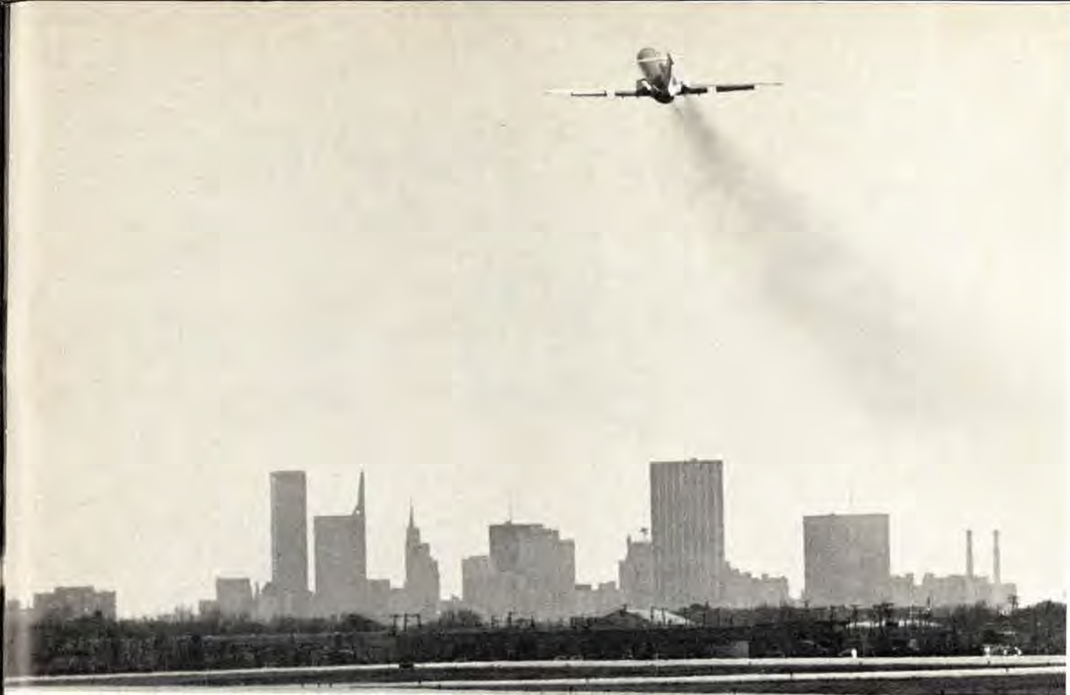
Climbing over the Dallas skyline, a tri-engine 727 jetliner illustrates the airlines' campaign to stop smoking—and polluting the air. The left engine runs clean with a new burner can; the right and center engines will soon be modified with the new equipment.
