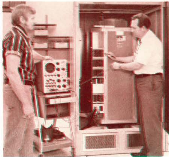
Weather messages destined for nationwide distribution are temporarily stored in a high-speed magnetic drum. WMSC computer technicians Bob McCall (left) and Walter Ray check over its circuit cards.
