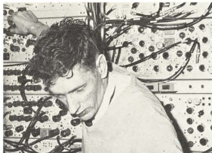
RADAR CERTIFICATION —Measuring and aligning the frequency handpass of a radar receiver, Technician Eugene O'Sullivan of Airway Facilities Sector 377 at Washington National Airport reflects the skill and concentration that recently won him a Quality Within Grade Pay Increase from Eastern Region Director George Gary.
