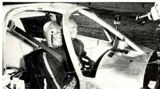
High-speed motion pictures (at 500 frames per second) record tests of several configurations for occupant restraint of belts and harnesses proposed for general aviation fliers. Dummies in fuselage are catapulted to a stop at .25 Gs in aviation safety studies.
