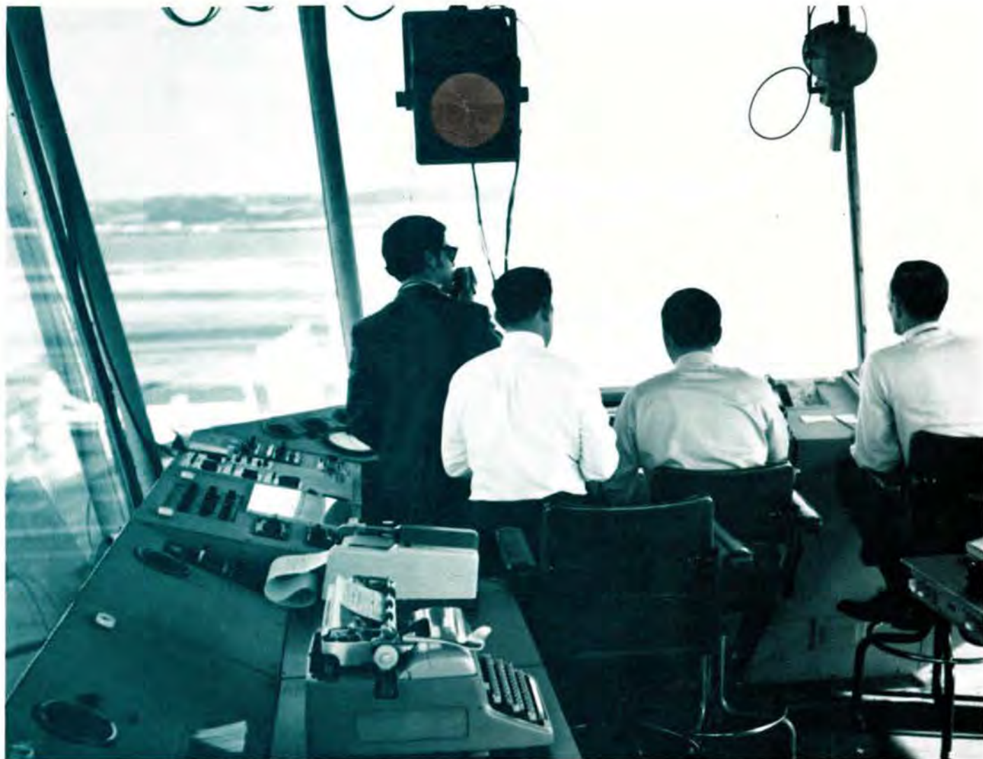
At Washington National, controllers can quickly scan the BRITE (Bright Radar Equipment—Tower Equipment) screen, which can be seen clearly even in a well-lit tower cab. The screen, which can be utilized to provide return from equipment like the new ASR-7 surveillance radar, is mounted on an overhead rail which can be moved as needs dictate.
