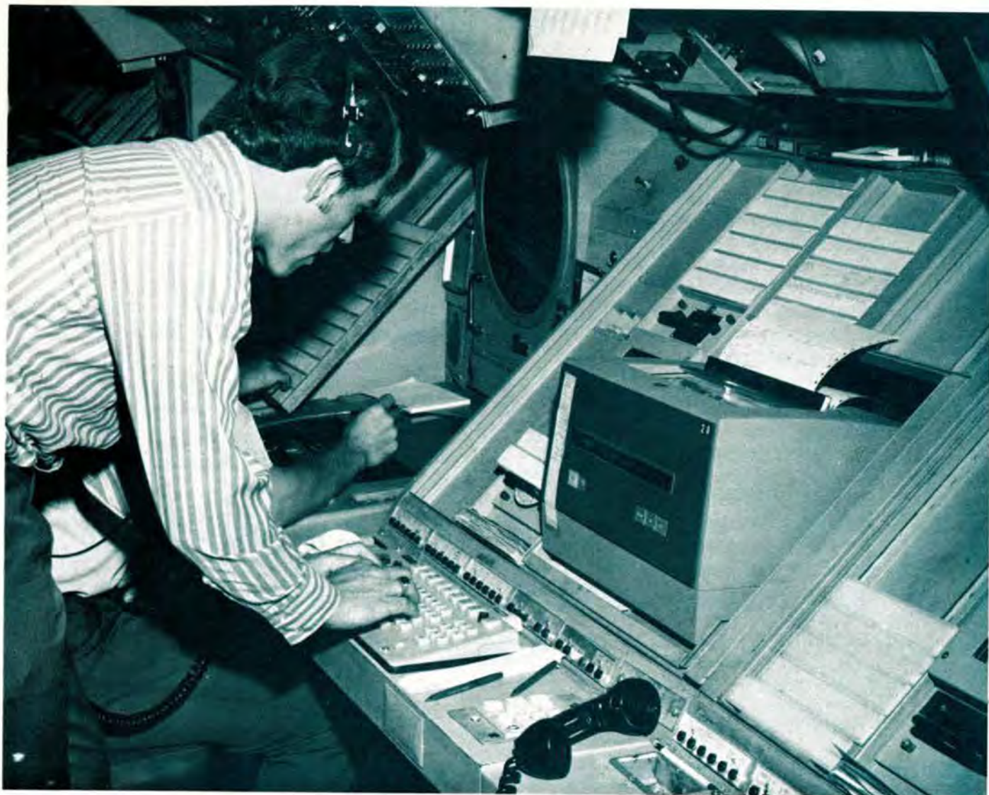
At Indianapolis, a controller double checks the content of a flight strip, using a keyboard that is part of CUE-Computer Update Equipment. Directly in front of the controller is the high-speed printer that produces new or changed flight information strips.
