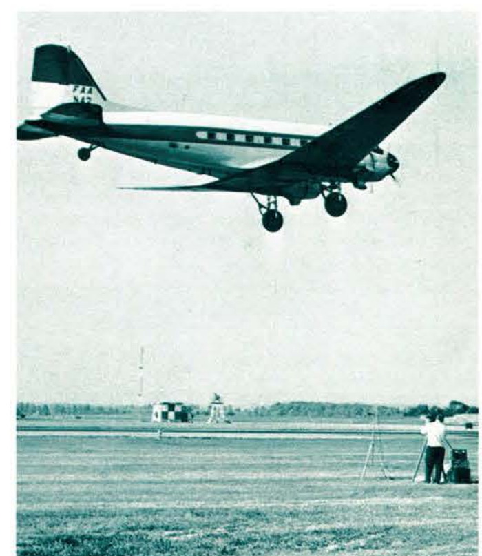
As agency DC-3 makes a low pass over runway, plane's exact position is checked through theodolite operated by team member Alex Friedman.
