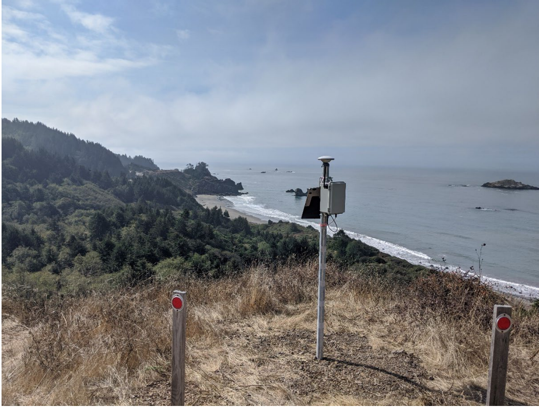
Figure C-6: Photograph of the base RTK-GNSS station at Hooskanaden looking south overlooking the bottom portion of the landside.
