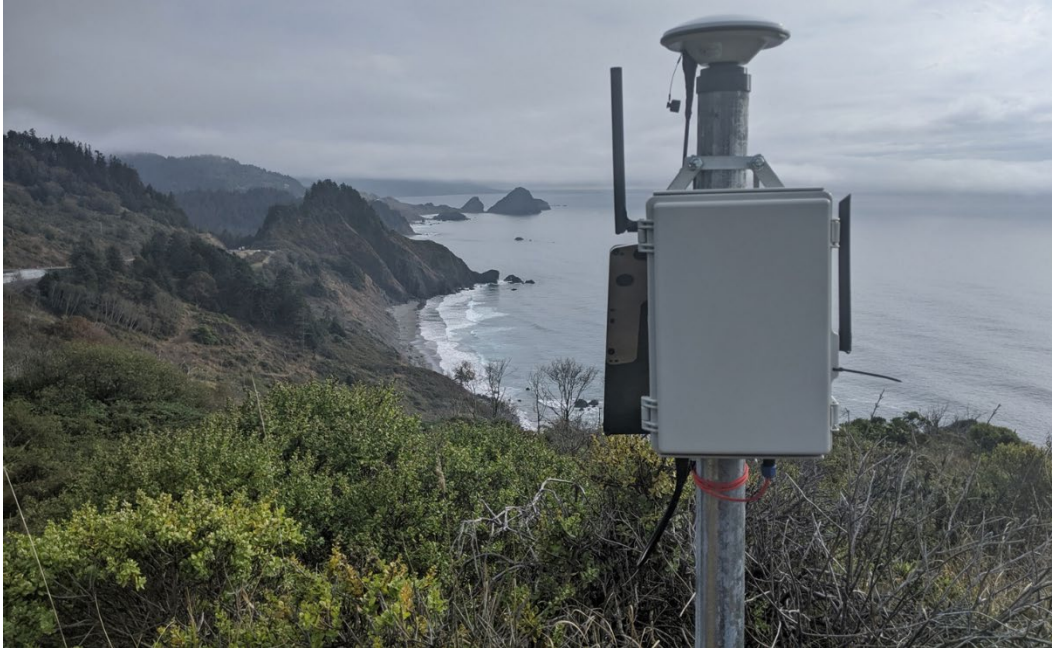
Figure C-4: Photograph of the base RTK-GNSS station at Arizona Inn overlooking the rest of the landside to the south.
