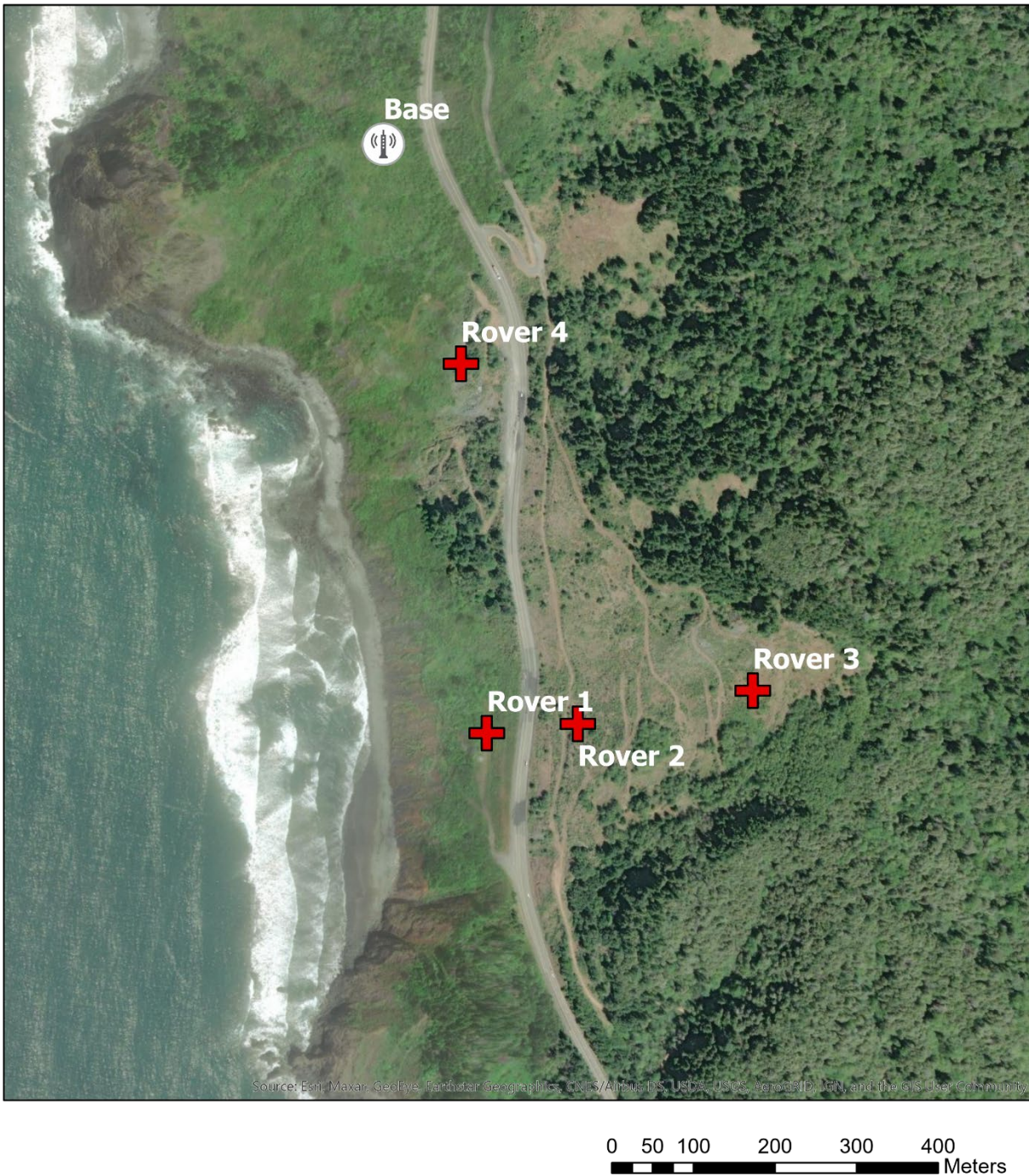
Figure C-3: Map of the Arizona Inn Landslide showing the location of the RTK-GNSS base and rover stations.
