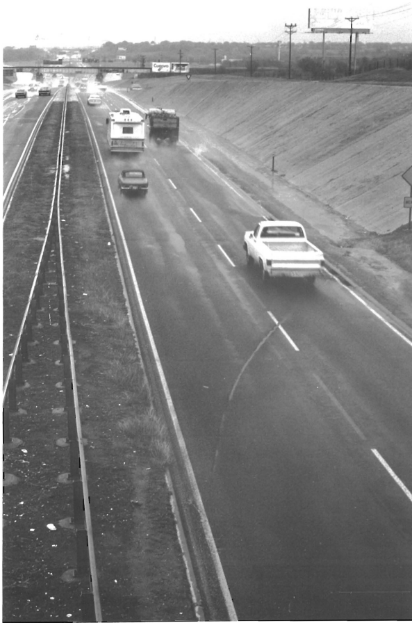
Figure 10. Splash and Spray Behind Automobiles in 0.02 in/h Rainfall; Location: 820/812/L,M,R,S 11/8/77
