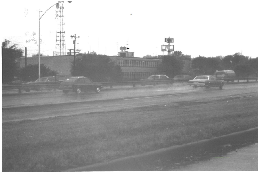
Figure 12. Splash and Spray Behind Automobiles in 0.04 in/h Rainfall K_{avg} = 0.014 ; Location: 30/1681/R&S
