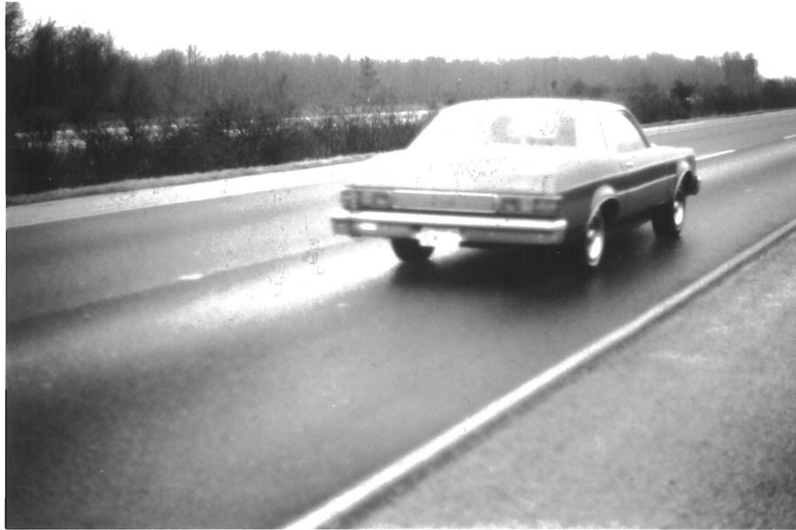
Figure 15. Splash and Spray Behind Automobile in 0.25 in/h Rainfall K_{avg} = 0.15 ; Location: 10/7392/L 2/9/78
