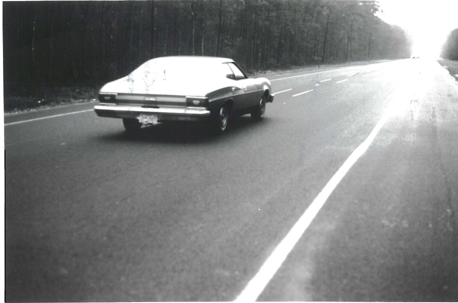
Figure 19. Splash and Spray Behind Automobile in 0.05 in/h Rainfall K_{avg} = 0.07 ; Location: 87/3057/L&R 2/9/78
