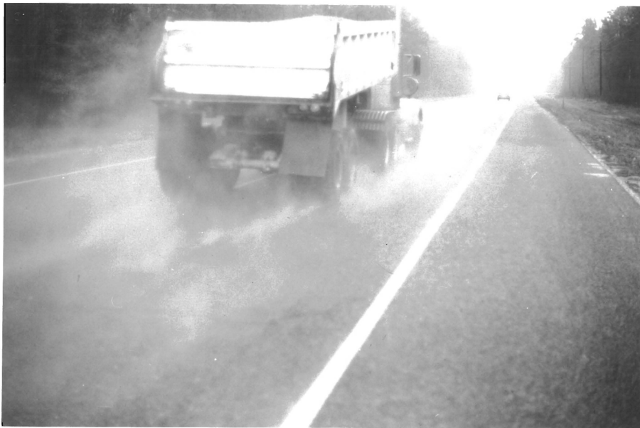
Figure 22. Splash and Spray Behind Truck in 0.06 in/h Rainfall K_{avg} = 0.011 ; Location: 87/3056/R&L 2/9/78
