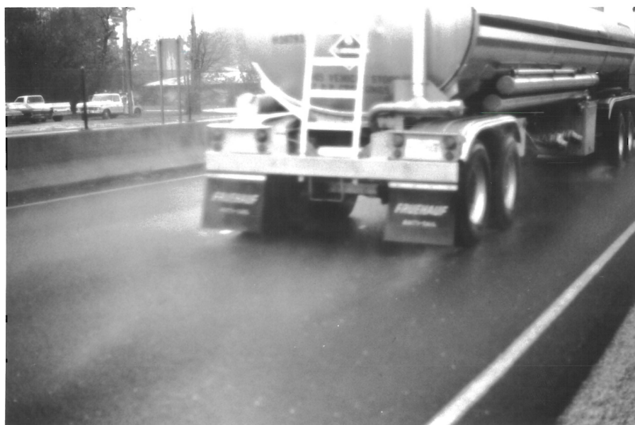
Figure 18. Splash and Spray Behind Truck in 0.25 in/h Rainfall K_{avg} = 0.11 ; Location: 10/289/R 2/9/78
