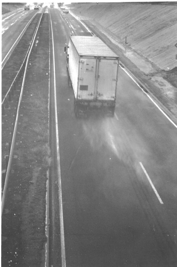
Figure 11. Splash and Spray Behind Truck in 0.02 in/h Rainfall; Location: 820/812/M 11/8/77
