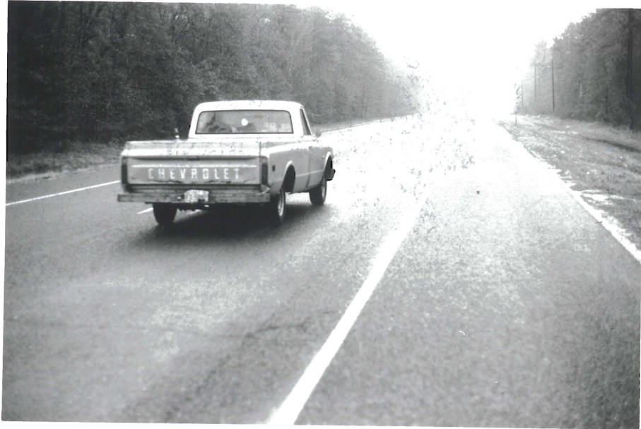
Figure 21. Splash and Spray Behind Pickup in 0.05 in/h Rainfall K_{avg} = 0.011 ; Location: 87/3056/R&L 2/9/78
