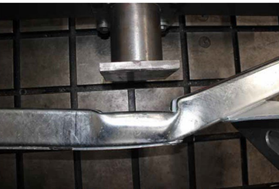
Figure 19. Images of post-test deformation in the P3 impact case comparing experimental results to simulation results for the Manac guard
