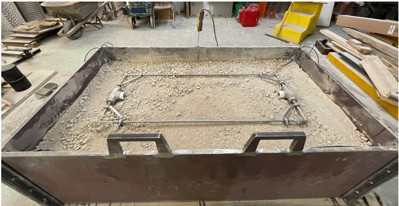
Figure 18. Photo. Large-scale test bed showing a field BE sensor installed within an aggregate layer.
