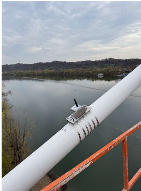
Figure 3 – Accelerometer Installed on a Stay Cable
