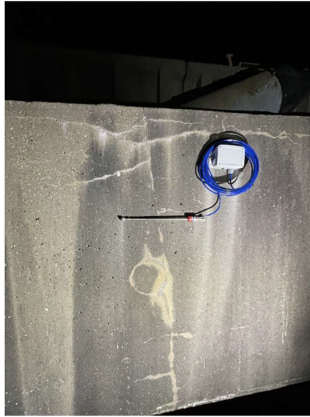
Figure 8 – Crackmeter Placed at Existing Crack
