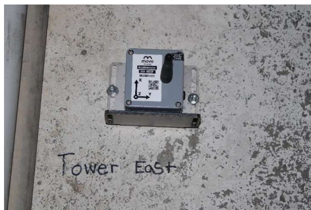
Figure 4 – Accelerometer Installed on Bridge Tower
