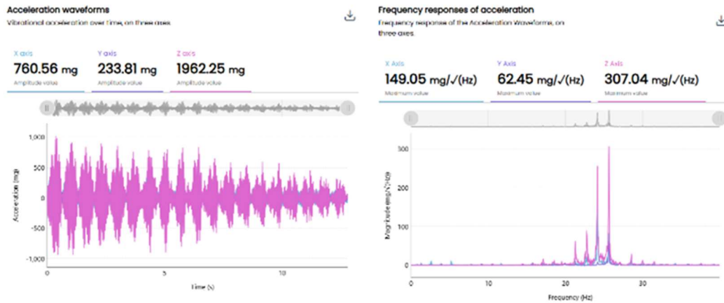
Figure 19 – Cable W12 Acceleration Response and FFT Under 20+ mph Wind Conditions Indicating VIV
