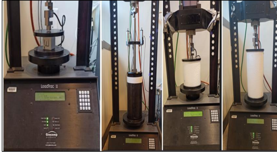
Figure 4. Example Setups Used to Conduct Unconfined Compressive Tests with Expanded Polystyrene
