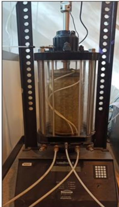
Figure 9. Cyclic Test Setup with Compacted Aggregate.
