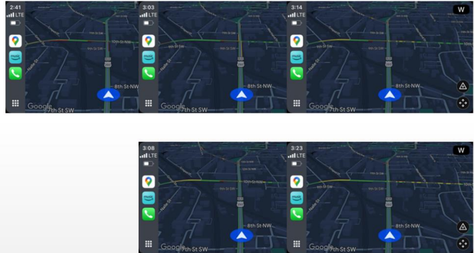
Figure 4. Alert Delivery for Low Bridge Warning at Downtown Charlottesville, Virginia
