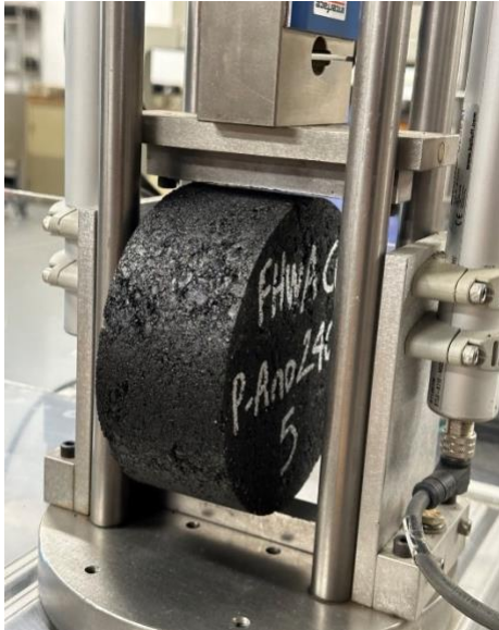
Figure 7: The IDEAL-CT Setup
