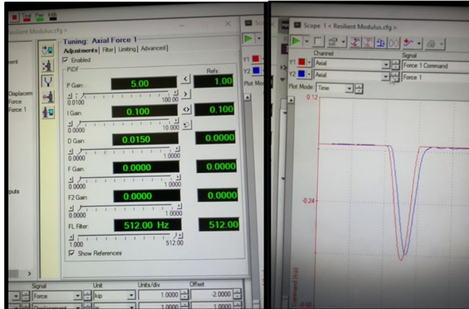
Figure 3.7. PIDF gains adjustment for haversine-shaped load pulse waveforms
