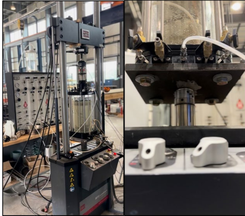
Figure 3.6. MTS Servo hydraulic Bottom-Loading test machine with its customized steel plate during M_R testing
