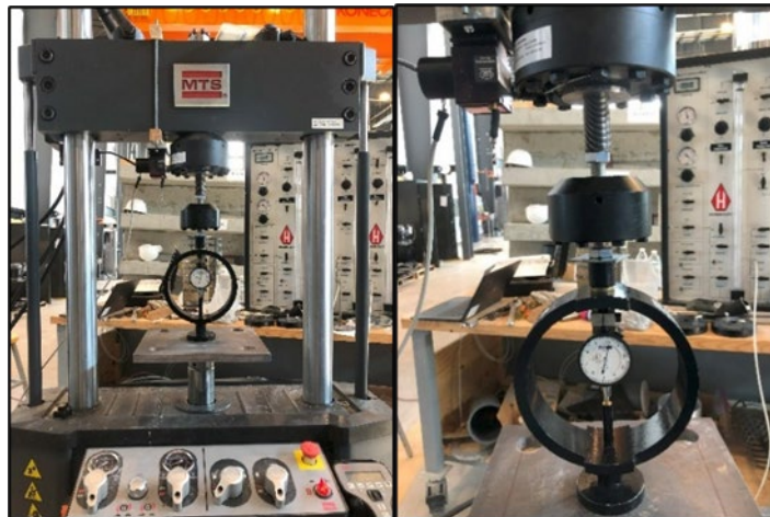
Figure 3.8. Load cell calibration with proving ring
