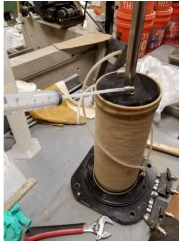
Figure 2.5. Injecting additional water into the specimen compacted at OMC (Ullah and Tanyu, 2020)
