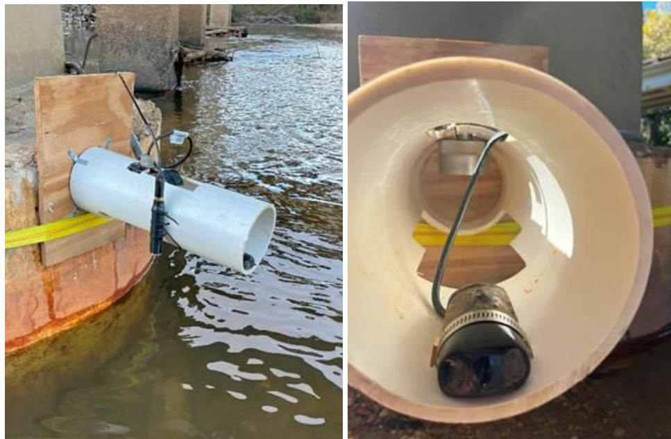
Figure 55. Installation of sensors: Sonar and turbidity sensors are placed facing the streambed, and the AV sensor is facing the upstream flow.
