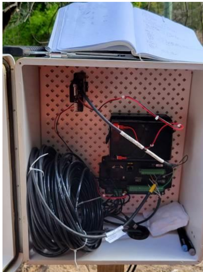
Figure 69. BIN 013310, Goshen, AL. Enclosure containing the data acquisition system and battery.
