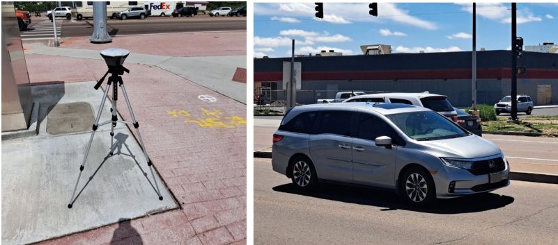
Figure X+T (a) Emlid RS+ base GNSS unit set up near the test site. (b) Test Vehicle driving through the intersection recording ground truth data while receiving differential correction through the base unit.
