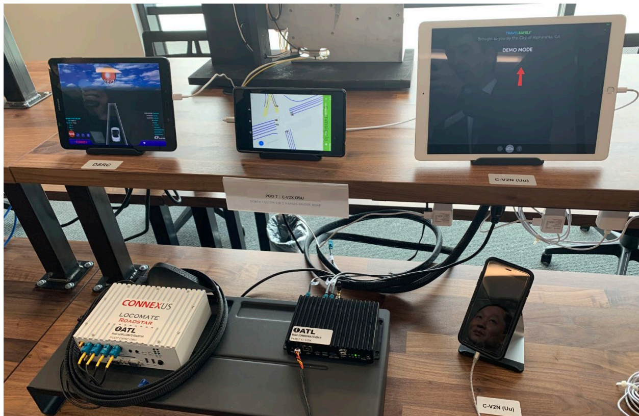
Exhibit 2. Connected vehicle hardware including DSRC OBU and HMI (Left), C-V2X OBU and HMI (Middle), and C-V2N (Uu) HMIs (Right)
