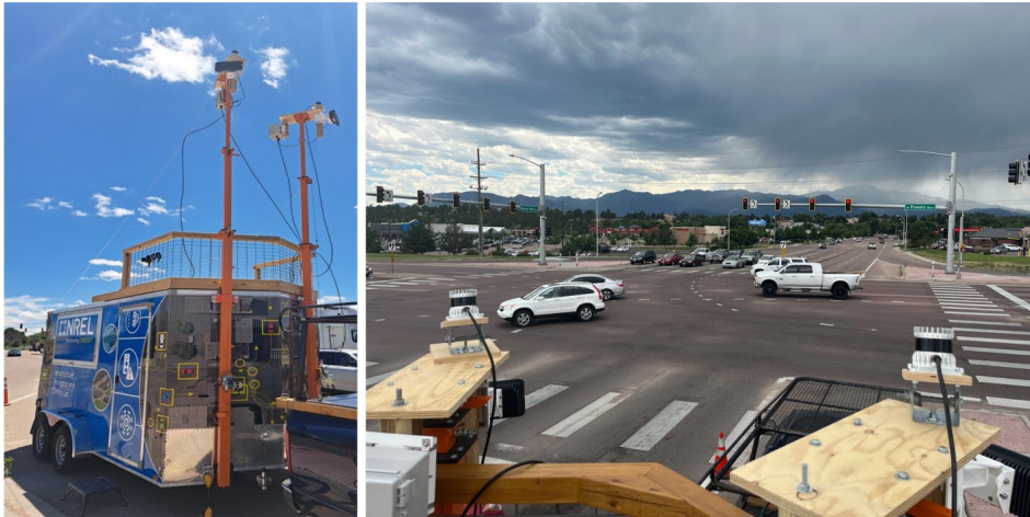
Figure 3 (a) The IPC mobile trailer deployed at the intersection with radar and lidar mounted on each extendable mast. (b) The intersection as seen from the top of the IPC mobile trailer.
