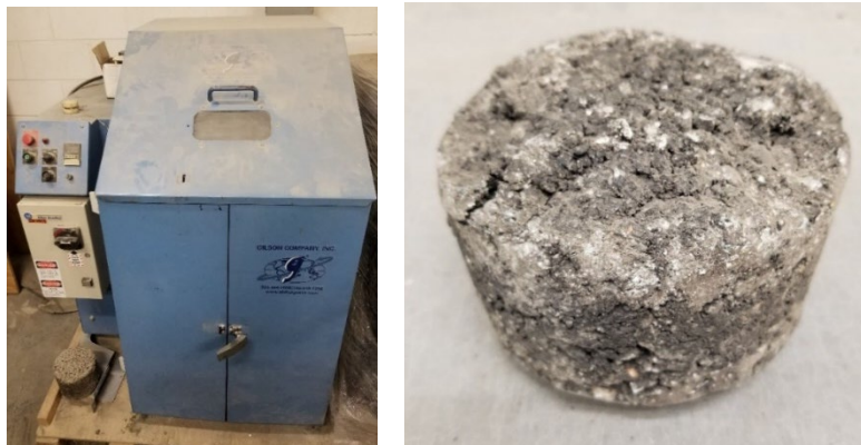
Figure 21. LA Abrasion Machine for Cantabro Testing (left) and Post-testing Cantabro Specimen (right)
