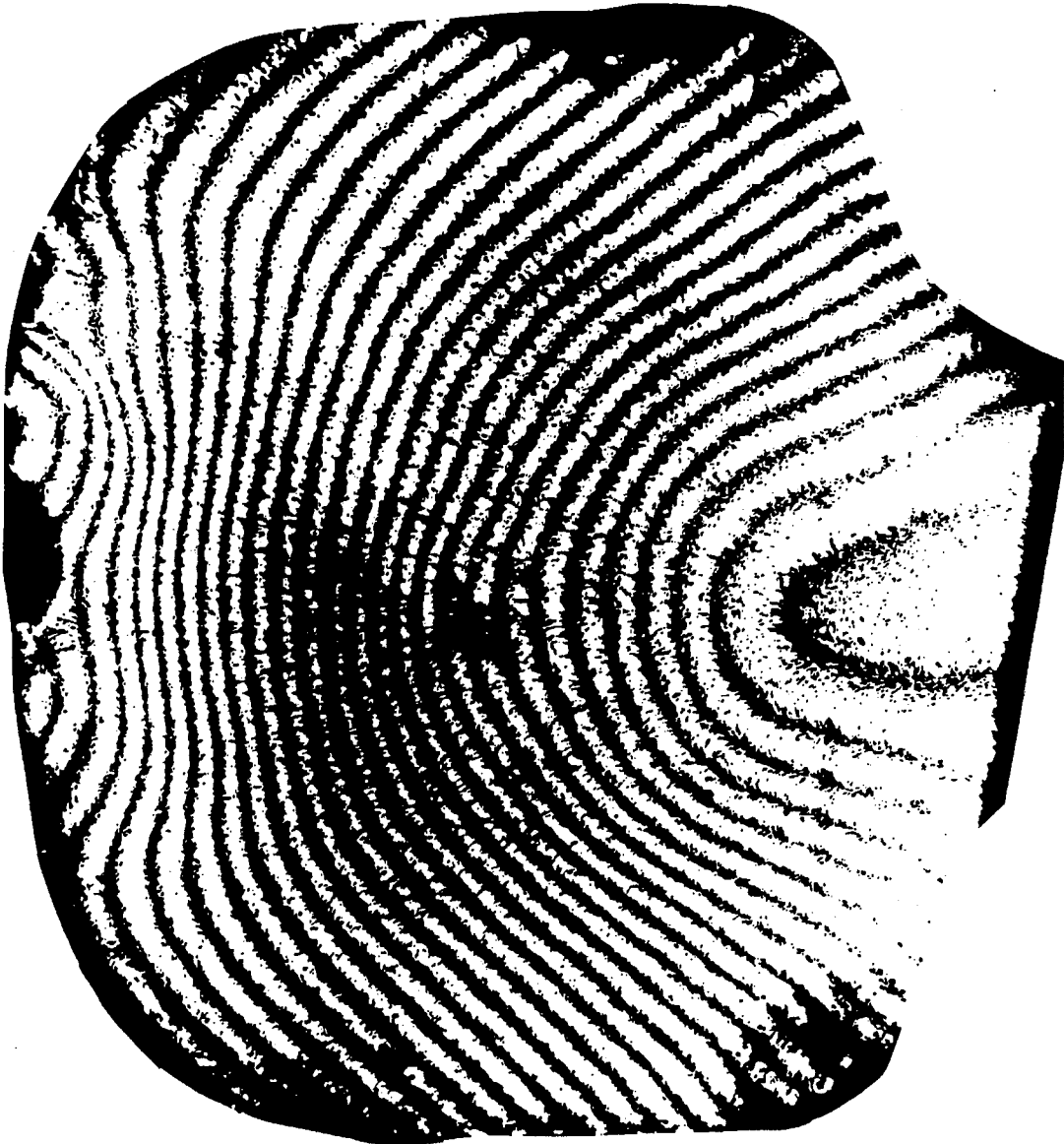
Fig. 65 v-field fringes by moiré interferometry (rail # 5 new CFI, 45° oblique slice)
