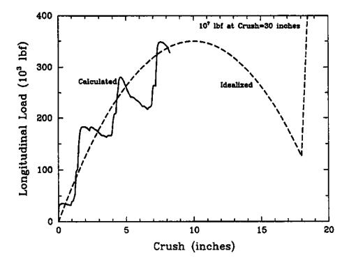
Figure 3-10. Calculated and Idealized Load-Crush Curves for the Baseline Anticlimber for Longitudinal Loading
