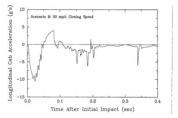
Figure 4-8. Lead Overridden Locomotive Crash Pulse Predicted for Scenario B, 30 mph Closing Speed
