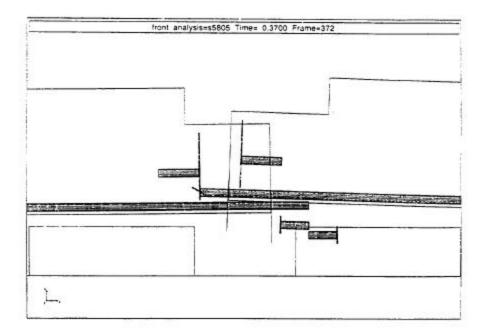
Figure 4-12. ADAMS View of the Front End Interaction at the Point of Maximum Lead Locomotive Crush for Scenario C, 43 mph Closing Speed
