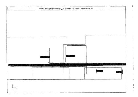
Figure 4-7. ADAMS View of the Front End Interaction at the Point of Maximum Lead Locomotive Crush for Scenario B, 30 mph Closing Speed
