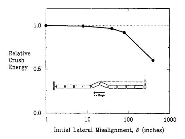
Figure 3-6. Collision Energy Dissipated in the Lead Locomotive as a Function of Lateral Displacement for a Coupler Connection
