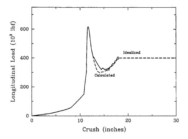
Figure 3-14. Calculated and Idealized Load-Crush Curves for the Baseline Short Hood/Collision Posts Structure for Longitudinal Loading
