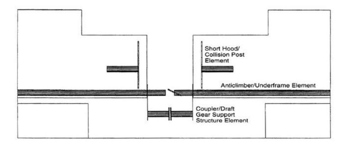
Figure 3-3. Locomotive Front End Impact Elements in ADAMS
