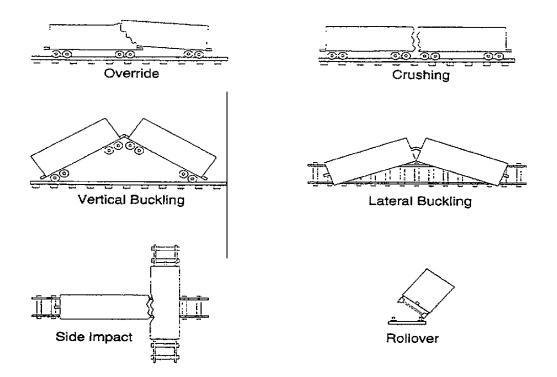
Figure 2-1. Possible Vehicle Collision Modes in Train Collisions
