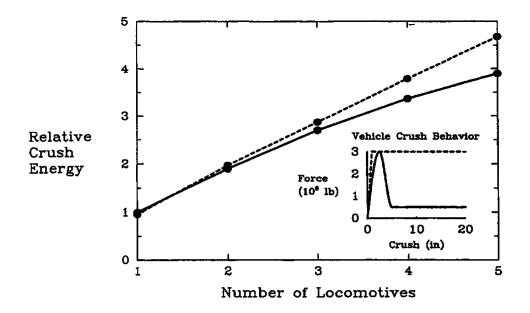
Figure 3-4. Collision Energy Dissipated in the Lead Locomotive as a Function of the Number of Trailing Locomotives of Equal Weight and Strength
