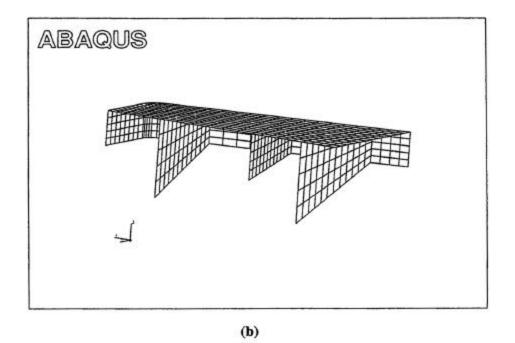
Figure 3-8. Finite Element Mesh Used in the Structural Damage Calculations of the Baseline Anticlimber (only one-half of the mesh is shown)
