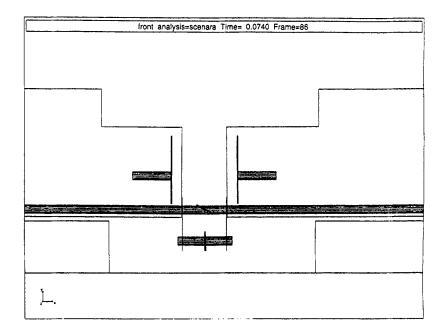
Figure 4-4. ADAMS View of the Front End Interaction at the Point of Maximum Lead Locomotive Crush for Scenario A, 18 mph Closing Speed
