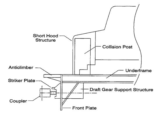
Figure 2-3. Illustration of a Road Freight Locomotive Front End
