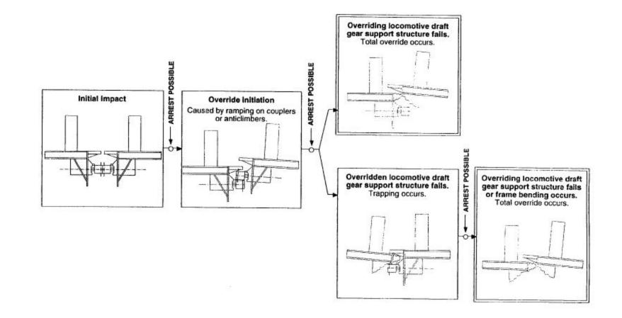
Figure 2-4. Two Potential Head-On Collision Override Sequences
