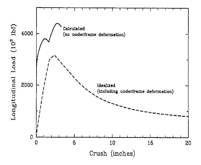
Figure 3-12. Calculated and Idealized Load-Crush Curves for the Baseline Draft Gear Support Structure for Longitudinal Loading
