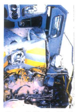
Figure 4-11. Front View Photograph of the Overridden Lead Locomotive in Scenario C, Showing the Limited Short Hood Structure Crush
