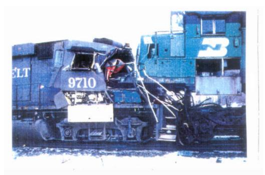
Figure 4-6. Photograph of the Override between the Two Lead Locomotives in Scenario B, 30 mph Closing Speed
