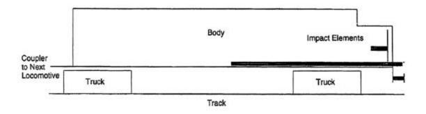
Figure 3-2. Locomotive Geometric Idealization Used in the ADAMS Model
