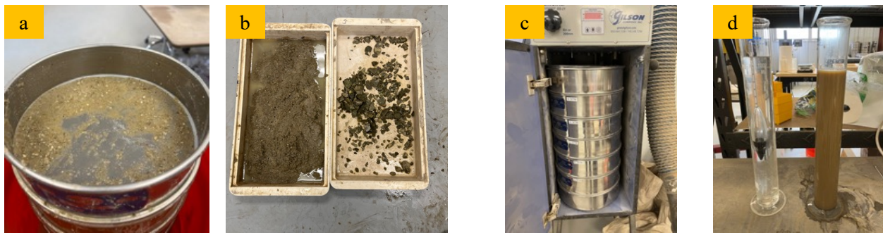
Figure 3.6 Sieve analysis: (a), (b) wet Sieving, (c) sieve shaker (dry sieving), (d) hydrometer test
