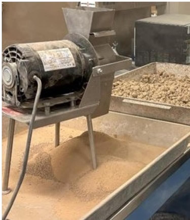
Figure 4.3 Grinding of soil lumps.
