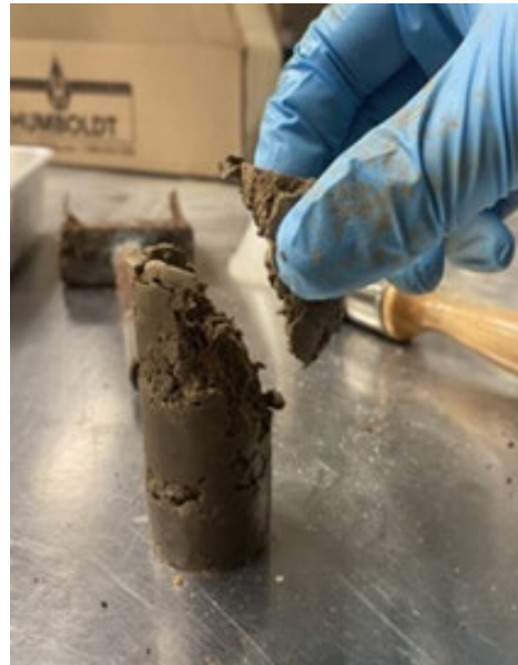
Figure 4.6 UCS sample after testing.
