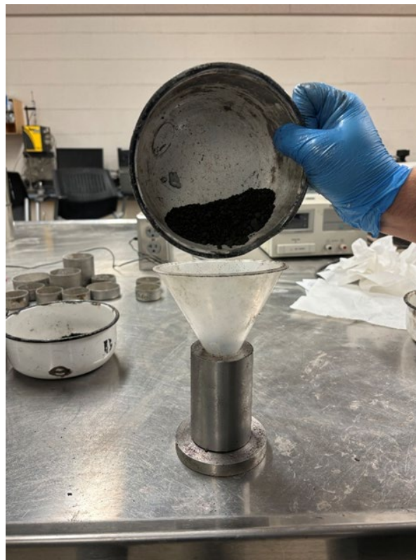
Figure A.6 Pouring Grey shale soil into the UCS mold for sample preparation and compaction.
