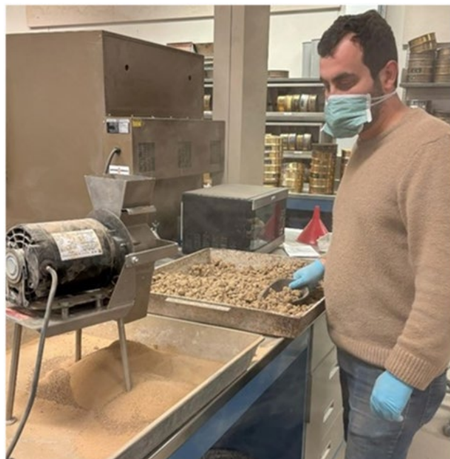
Figure A.2 Grinding clay soil.
