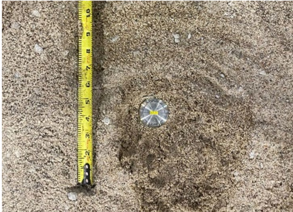
Figure 4.22 Pressure cell on compacted sand layer.
