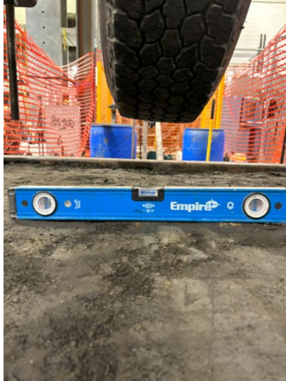
Figure A.17 Leveling the surface after compacting the second lift of the grey shale.
