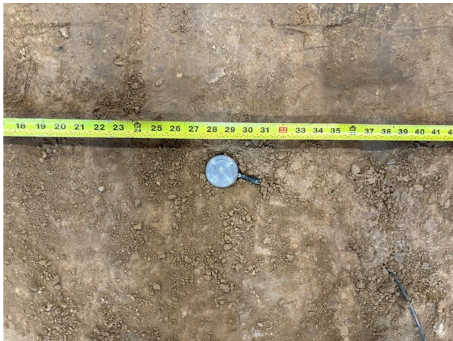
Figure 4.23 Pressure cell on compacted clay layer.
