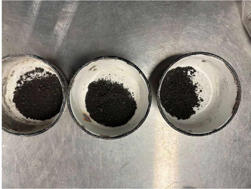
Figure A.5 Grey shale divided into three equal layers for consistent compaction and testing.
