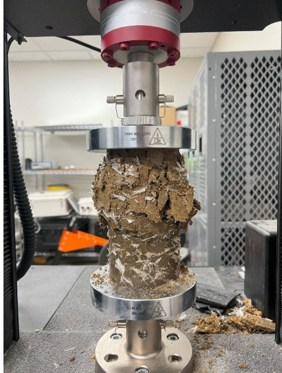
Figure A.13 Fiber-reinforced clay sample after testing.
