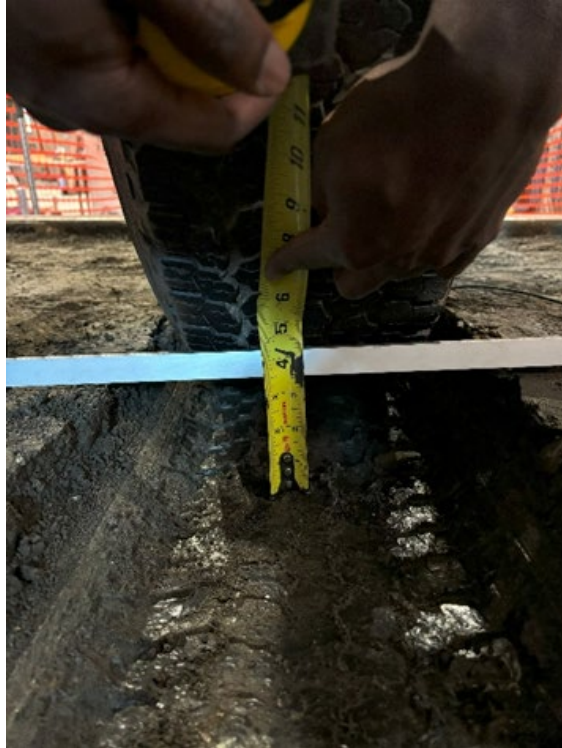
Figure A.19 Measuring permanent rutting depth using a tape measure after terminating the test on the grey shale base layer.
