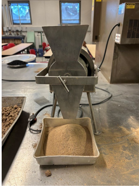
Figure A.3 Clay soil after grinding.
