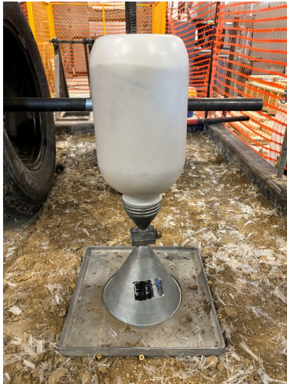
Figure A.22 Performing a sand cone test to measure the density of the compacted fiber-reinforced clay layer.
