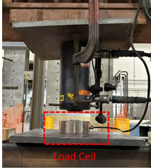
Figure 4.25 Load cell positioned beneath actuator.
