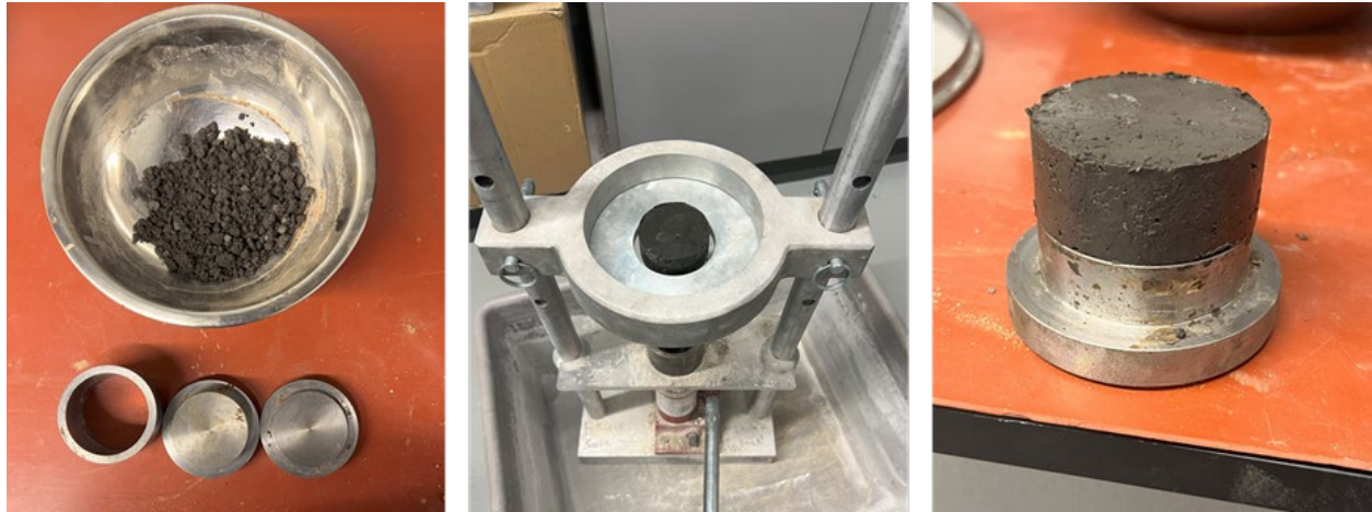
Figure 4.12 Soil mixing, specimen molding, and final compacted sample prepared for direct shear testing.
