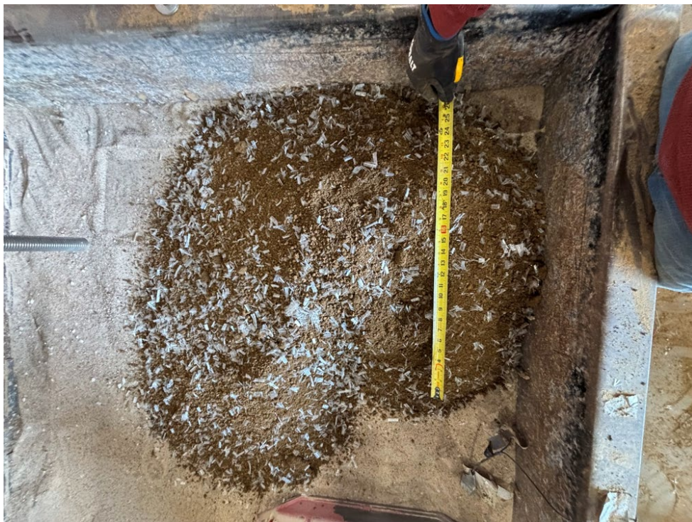
Figure A.20 Pour 0000the mixed fiber and clay soil to prepare the first lift of the fiber-reinforced clay base layer.
