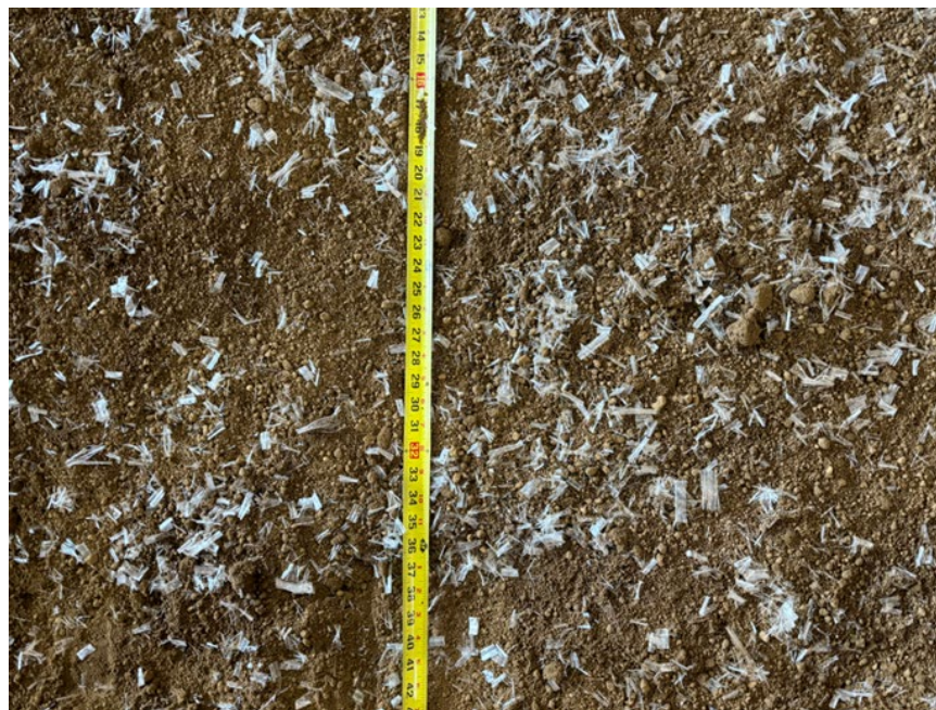
Figure 4.19 Compacted clay-fiber layer.
