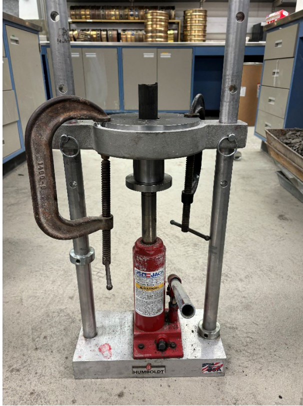
Figure A.7 Extracting UCS samples from the mold using a hydraulic jack.
