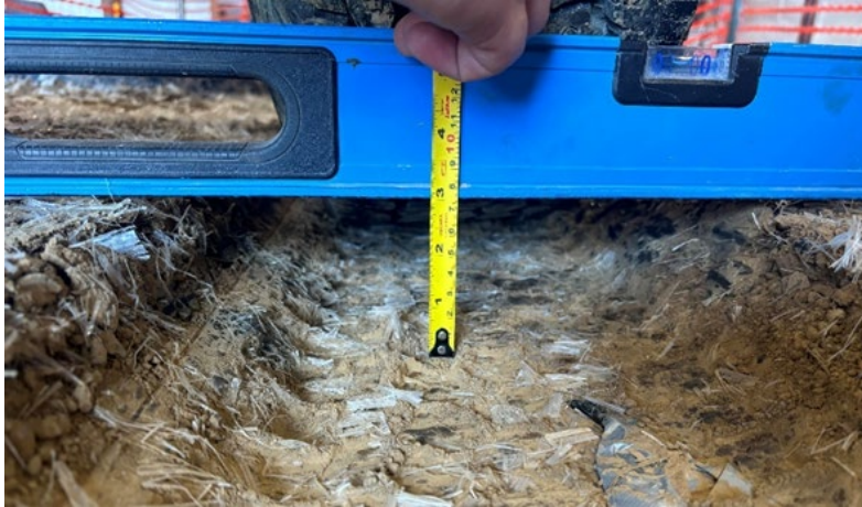
Figure 5.26 Rutting measurement using a measuring tape for the fiber-reinforced case.
