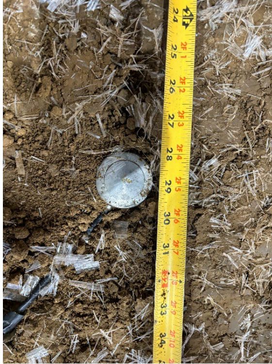
Figure A.21 Installing pressure sensors within the fiber-reinforced clay layer.
