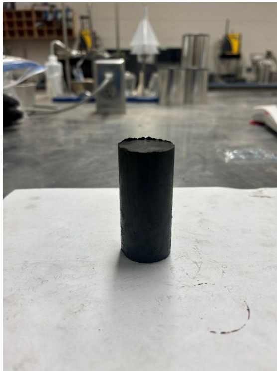
Figure A.8 Prepared UCS sample of grey shale soil, ready for UCS testing.
