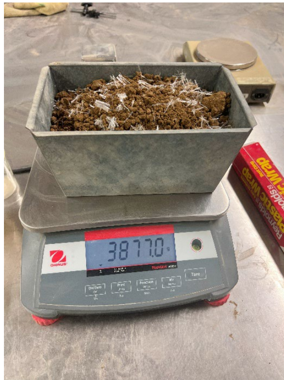
Figure A.10 Mixing clay soil with fiber reinforcement
