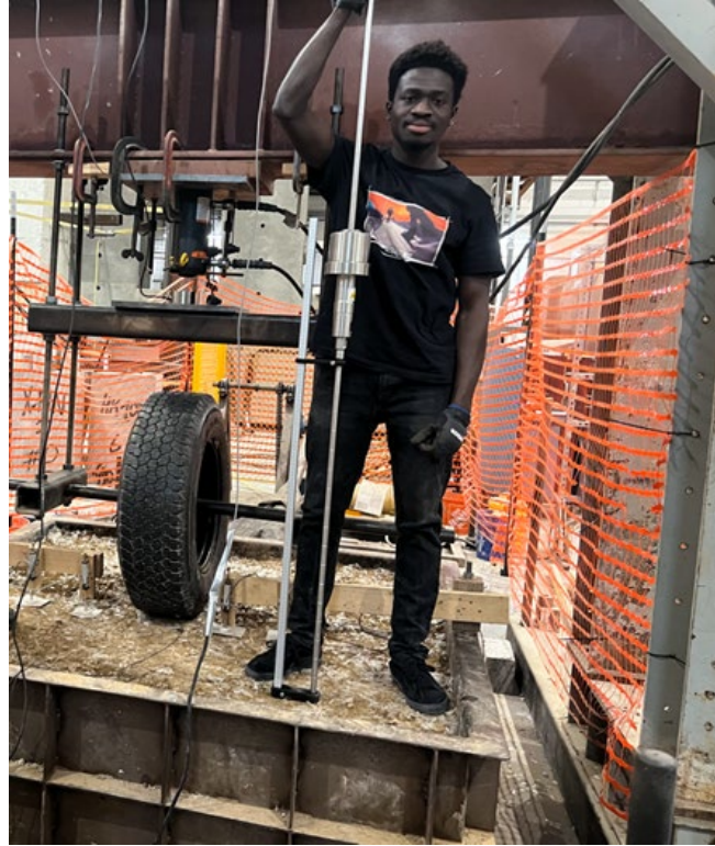
Figure 4.28 DCP test on compacted fiber reinforced clay layer.
