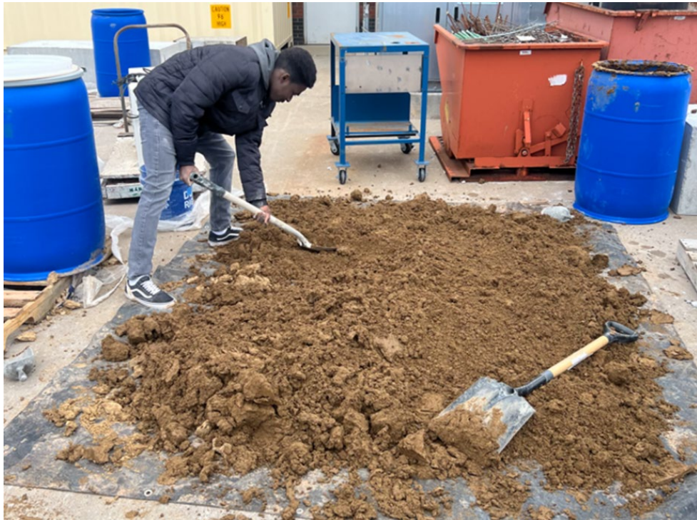
Figure A.1 Air drying the wet soil.
