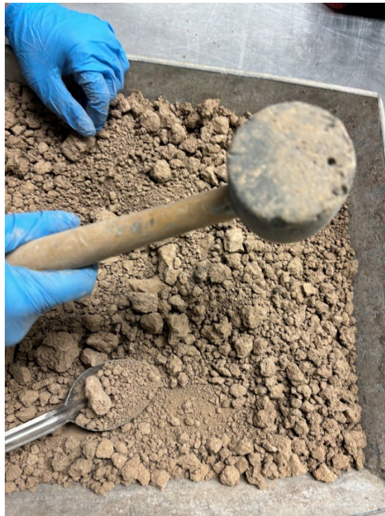
Figure A.4 Breaking down clay soil clumps using a rubber mallet to achieve finer particles for testing.
