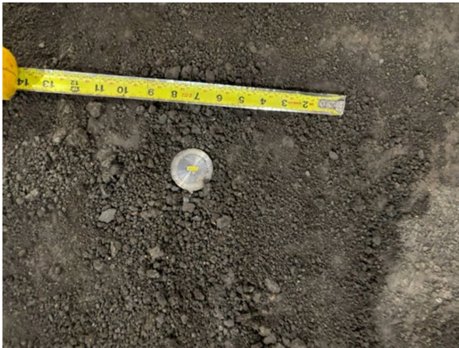
Figure A.16 Installing the middle pressure cell after compacting the first lift of the grey shale base layer to measure stress distribution.
