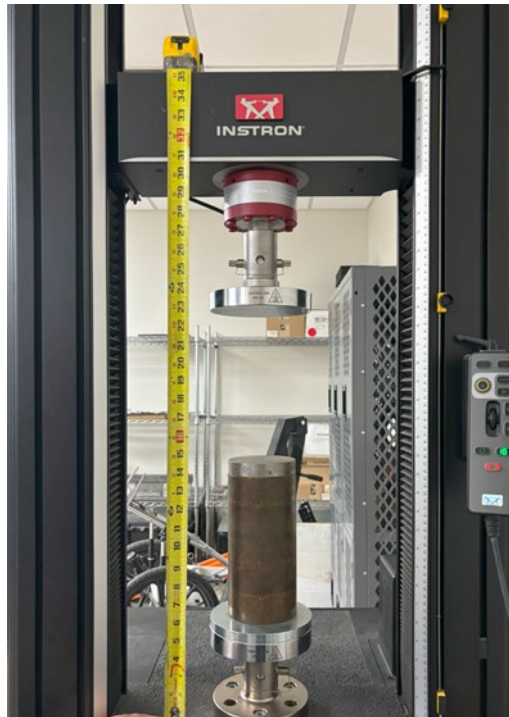
Figure 4.9 Instron testing device for fiber reinforced UCS.
