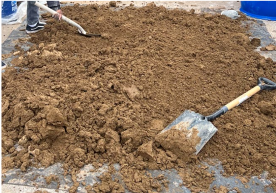
Figure 4.2 Air drying clay soil.
