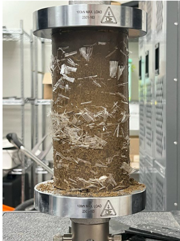
Figure A.11 Fiber-reinforced clay sample under the testing machine.
