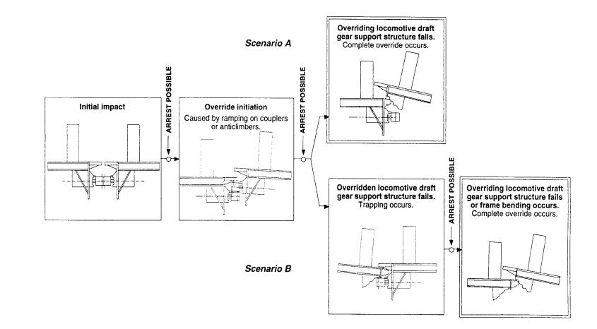
Figure 2. Two Potential Head-On Collision Override Scenarios
