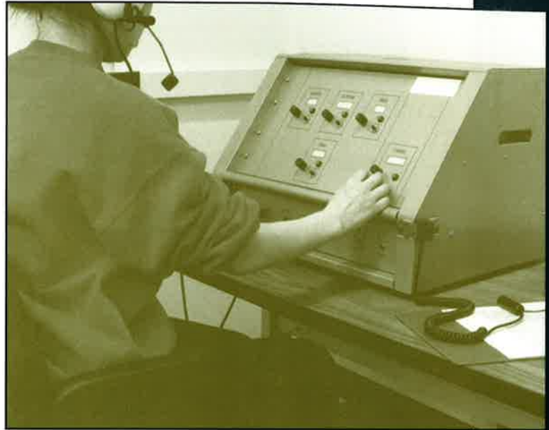
This simulated mode control panel helps Volpe Center researchers evaluate communication errors in controller-pilot transmissions.
