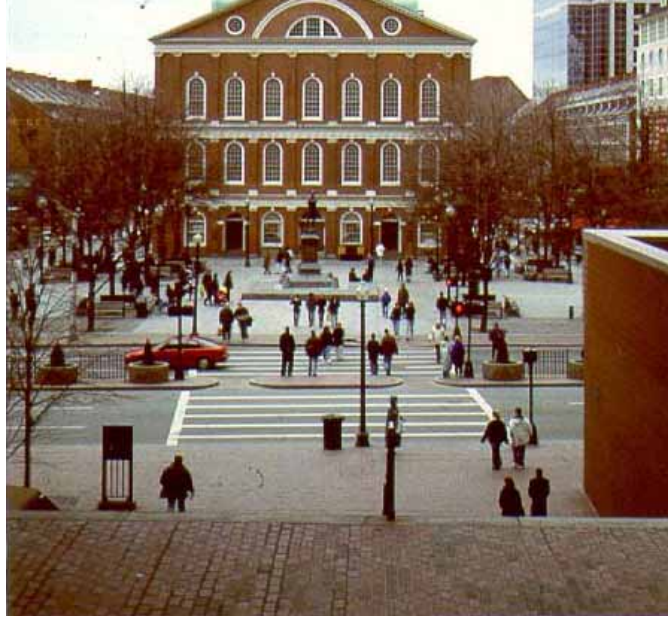
Figure 12-2. Photo. Refuge islands and visible crosswalks are essential on major arterials with higher traffic speeds.
