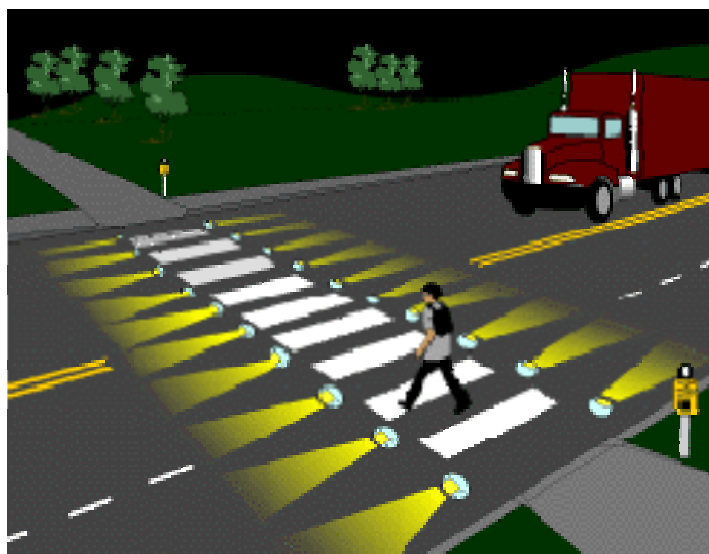
Figure 10-10. Illustration. Example of in-roadway warning lights.
