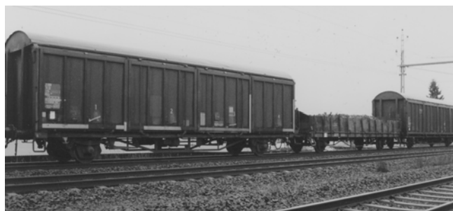
Figure 7: Freight train of mixed consist. Covered type Hbis wagons and open type Oms wagons.
