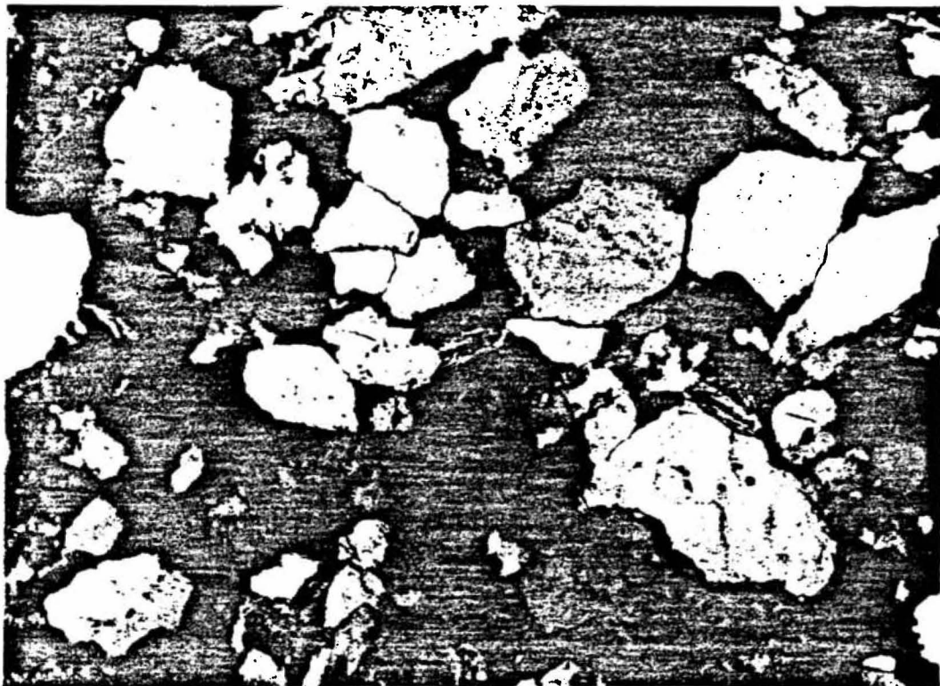
Figure 19 (X-40) Aggregate 4801, quartzite (x-polars).
