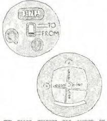
THE PILOT SELECTS HIS COURSE BY TURNING THE KNOB ON THE UPPER DIAL UNTIL THE NUMBERS ARE THE SAME AS THAT OF THE COMPASS BEARING OF THE STATION TO OR FROM WHICH HE WISHES TO FIX. ONCE THE COURSE IS SELECTED, THE PILOT KNOWS HE IS STAYING ON IT THEN THE VERTICAL NEEDLE ON THE LOW-ER DIAL POINTS DIRECTLY DOWNWARD.
