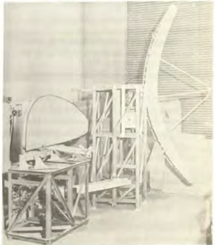
Azimuth and elevation antennae assemblies which pick up the signals of landing aircraft.
