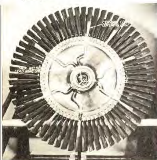
Figure 3. Turbine Wheel with Strain gauges to measure Vibration Frequency
