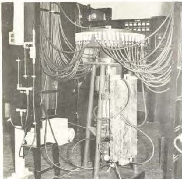
This is the Doppler distributor unit, nicknamed "Cream Separator" for obvious reasons.
