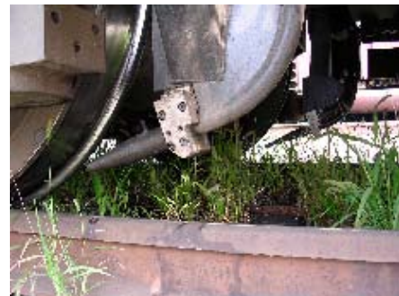
The fully computerized TracGlide system precisely applies lubricant to the tops of the rails.
