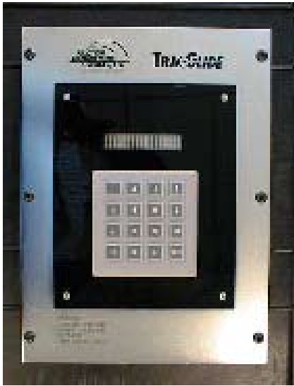
The TracGlide Computer is installed in the locomotive cab above the locomotive computer.
