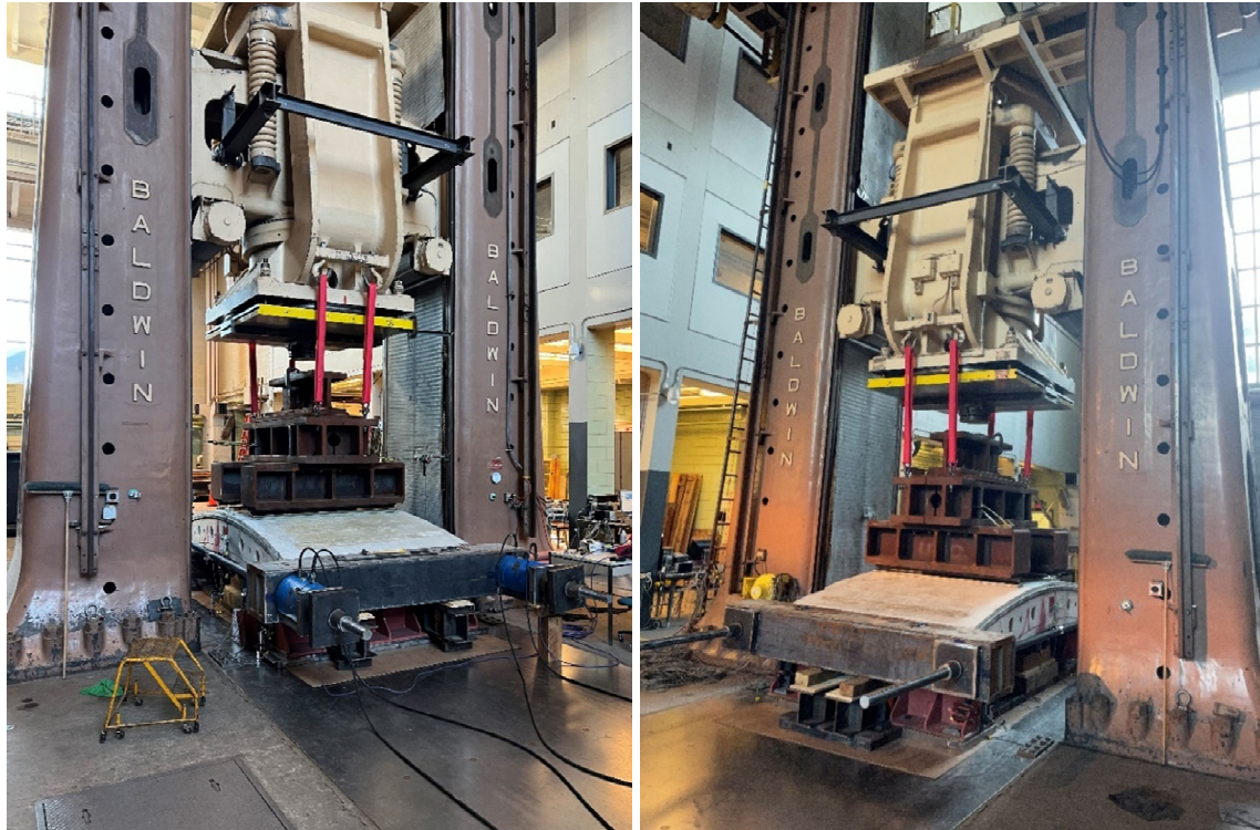
Figure 29: Radial joint test assembly: west side (left) and east side (right)
