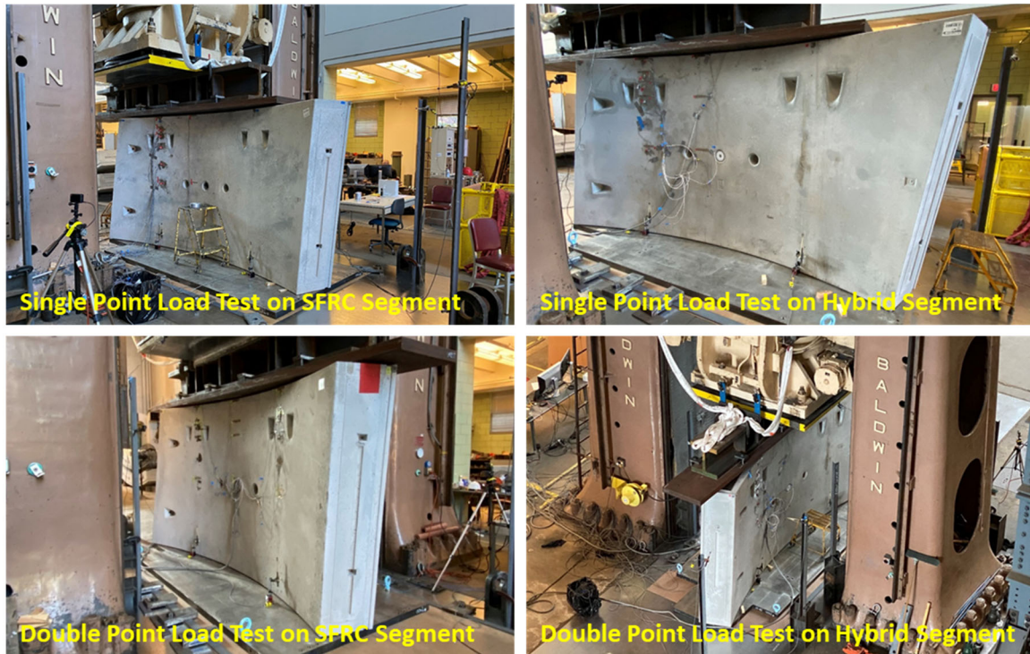
Figure 12: Test setups for thrust jacking load testing
