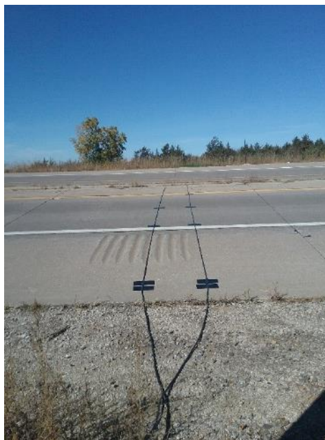
Figure 5.11: Tube Placement for Each Counter
