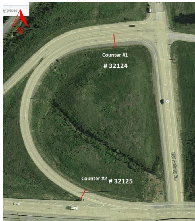
Figure 5.10: Road Tube Layout Used for Data Collection Source: Google (n.d.)
