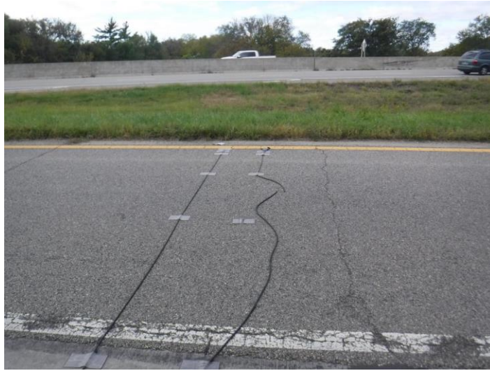
Figure C.13: Adams St North Counter 2, Broken Road Tube
