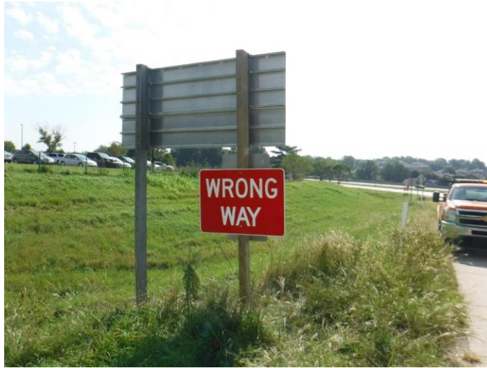
Figure C.17: Installation of 1st Oversized and Lowered Wrong Way Signs on Wanamaker Rd North Ramp
