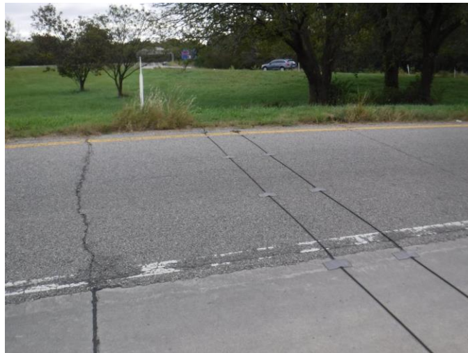
Figure C.12: Adams Street South, Later Discovered Road Tube Damaged
