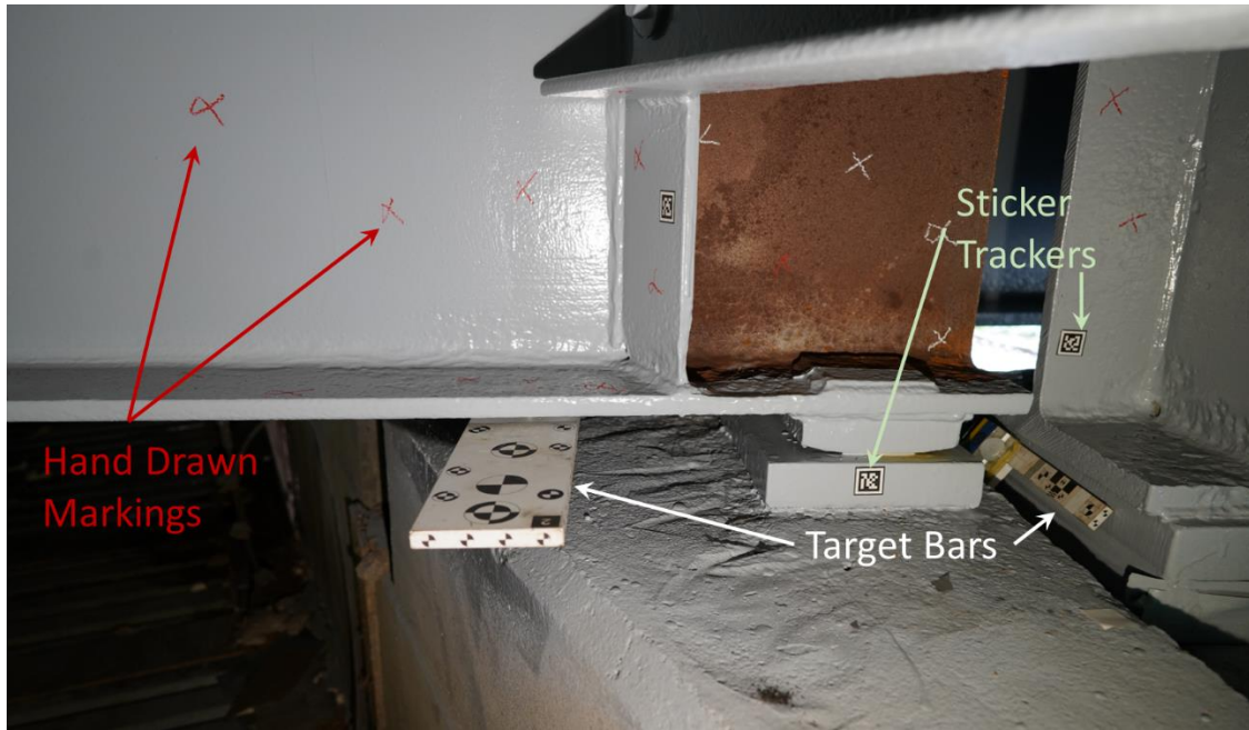
Figure 8. Representative views showing different tracking markers used for handheld scanning.
