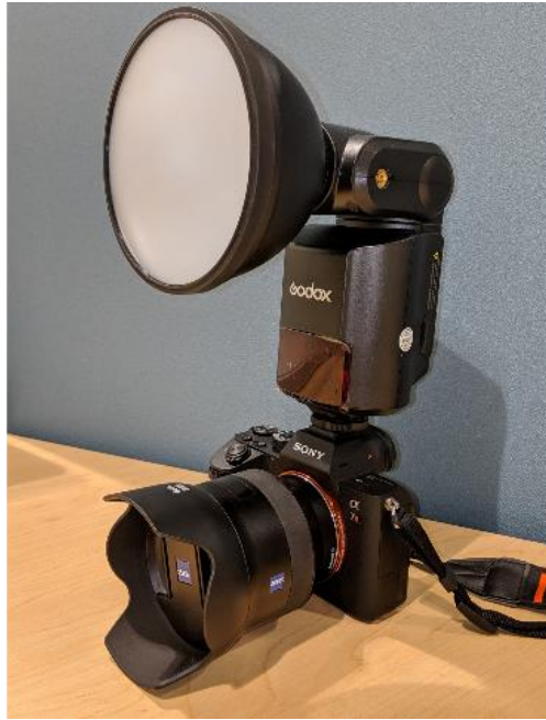
Figure 6. Equipment used for photogrammetry including the camera, lens and flash.
