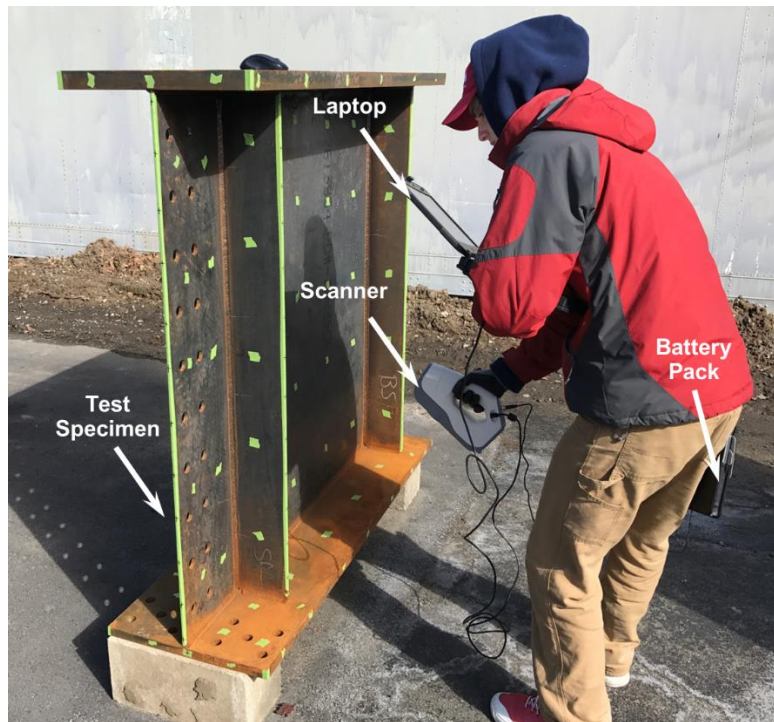
Figure 17. Scanning of beam end with simulated corrosion damage.
