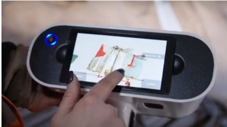
Figure 7. Representative view showing beam section scanned with Artec Leo in the field. Areas shown in red detail where information is missing.
