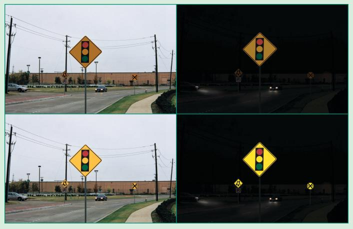
These photos demonstrate the improvement in visibility, during daytime and at night, made possible by using fluorescent yellow versus standard yellow signs. During the day and at night the fluorescent yellow signs (bottom) appear brighter than the standard yellow signs (top). *Photos: 3M.*
