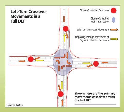
Administration (FHWA) study, *Alternative Intersections/Interchanges: Informational Report* (in preparation), used a traffic simulation model to compare throughput results for the following four DLT cases to those of conventional intersections: Case 1. Three lanes on the major road intersecting three lanes on the crossroad.
