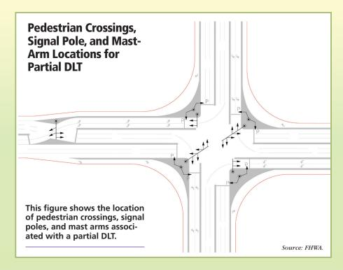
can build them in less time. At highvolume intersections, DLTs have the potential to reduce travel times considerably. Simultaneous movement of the left-turn and through traffic promotes improved progression of traffic platoons (moving of vehicles in groups where the vehicles are closely interspaced) on the arterial and increases vehicular throughput.
