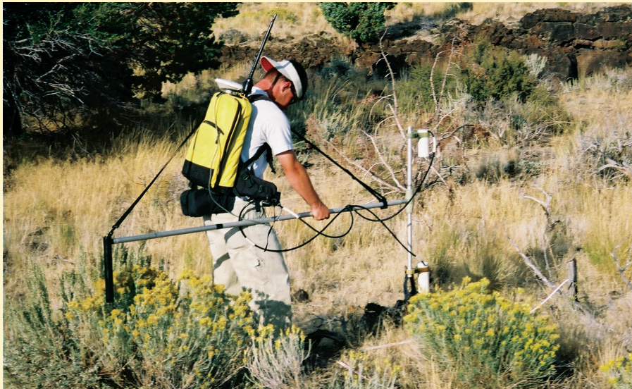
A worker uses a magnetometer to survey ground mass over known lava tube locations in Lava Beds National Monument, CA.
