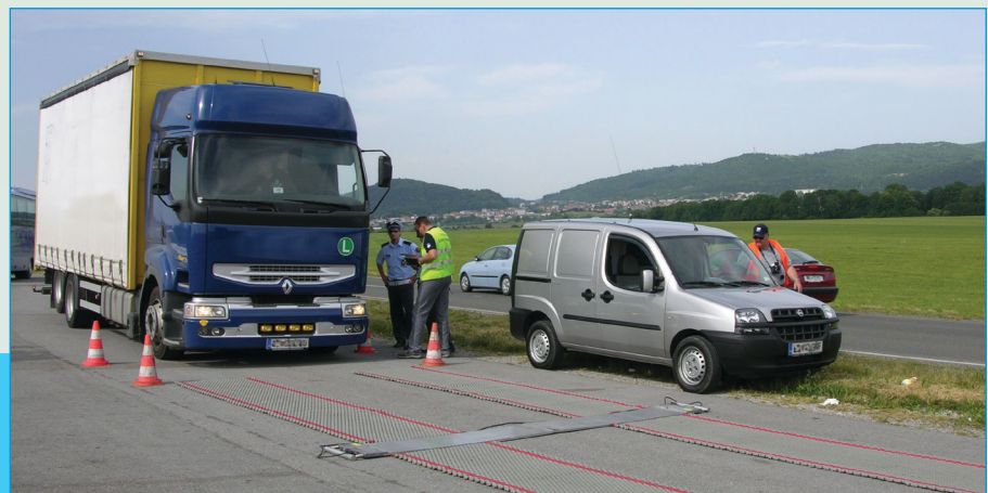
Portable static scales are weighing this truck at a mobile enforcement site in Slovenia.
