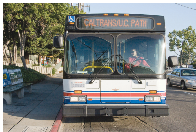
This Caltrans magnet-guided bus is precision docking at a bus stop during a demonstration run on State Route 185 in San Leandro, CA.
