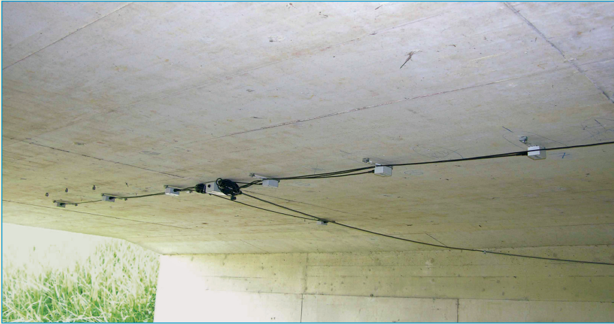
Shown here are strain gauge and data hub instrumentation for bridge WIM technology on the underside of a concrete bridge deck near Ljubljana, Slovenia.
