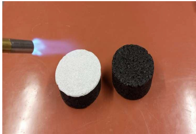
Figure 3.2: Application of Preformed Thermoplastic on Asphalt Surfaces
