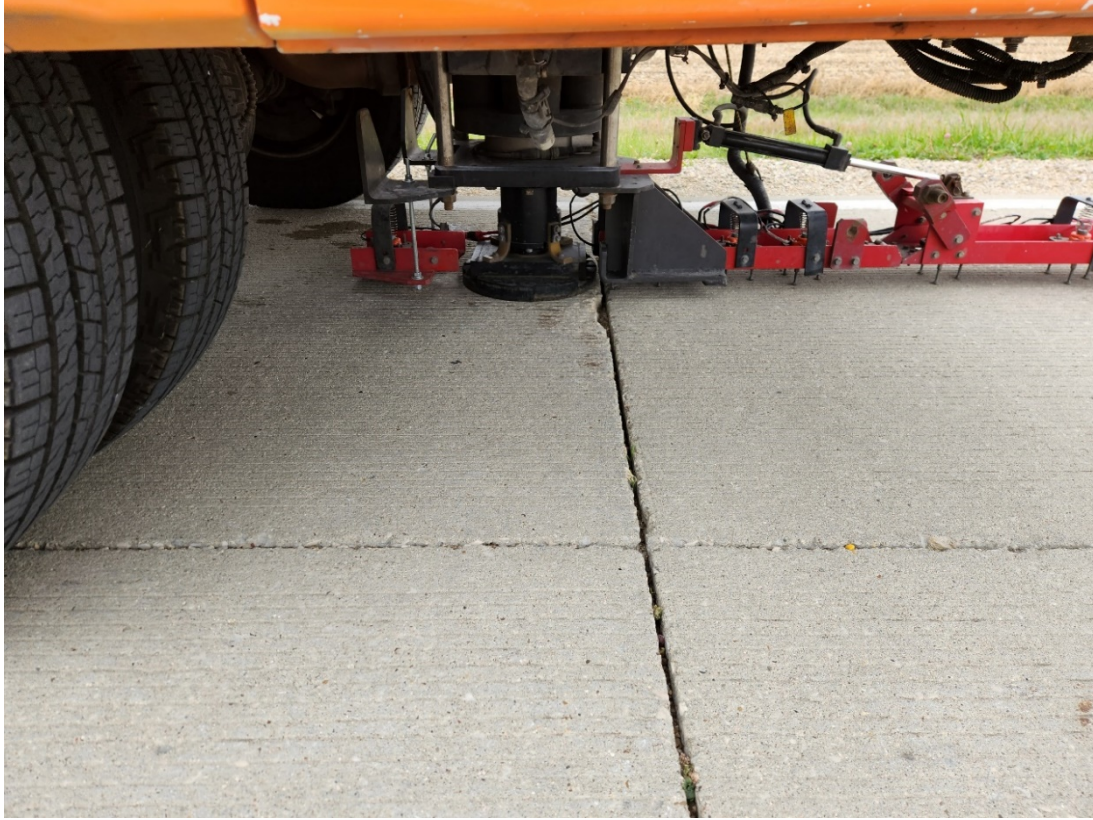
Figure 7. FWD test at a transverse joint
