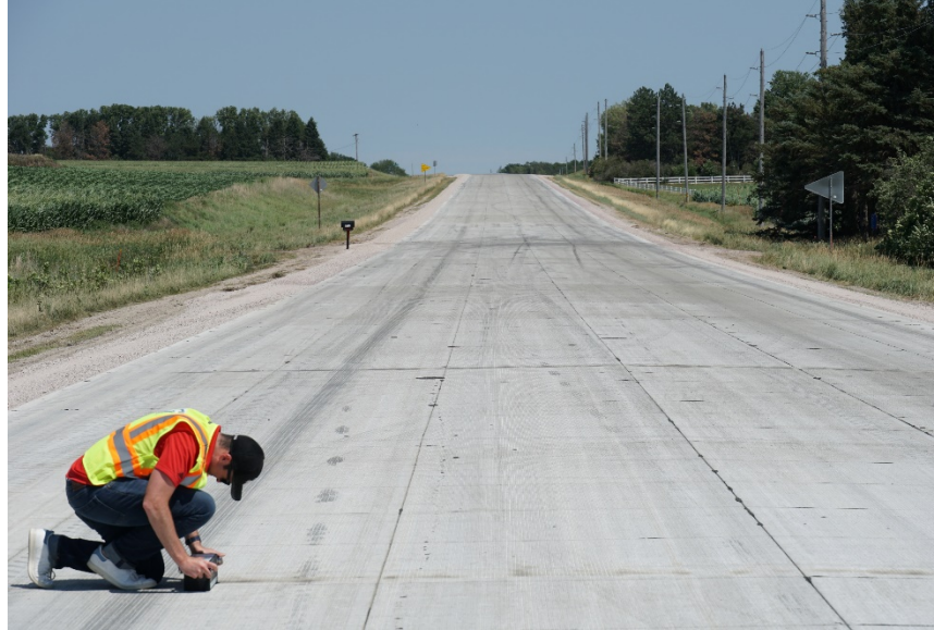
Figure 4. MIRA testing on a concrete pavement for joint activation
