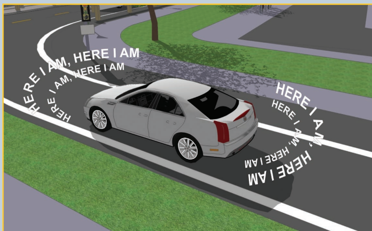
This illustration shows a vehicle broadcasting “Here I Am” messages as part of basic V2V communications.
