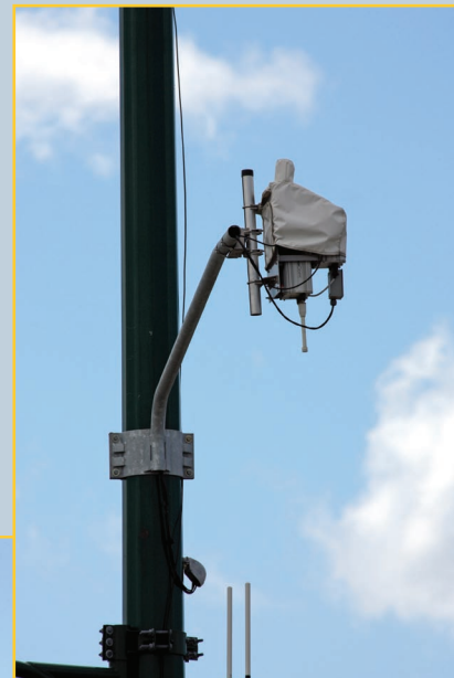
(Bottom) Shown here is the intersection test site in Oakland County, MI, used in the proof-of-concept test of 5.9 gigahertz dedicated short-range communications technology. (Right) A closeup of the prototype equipment used in the test.
