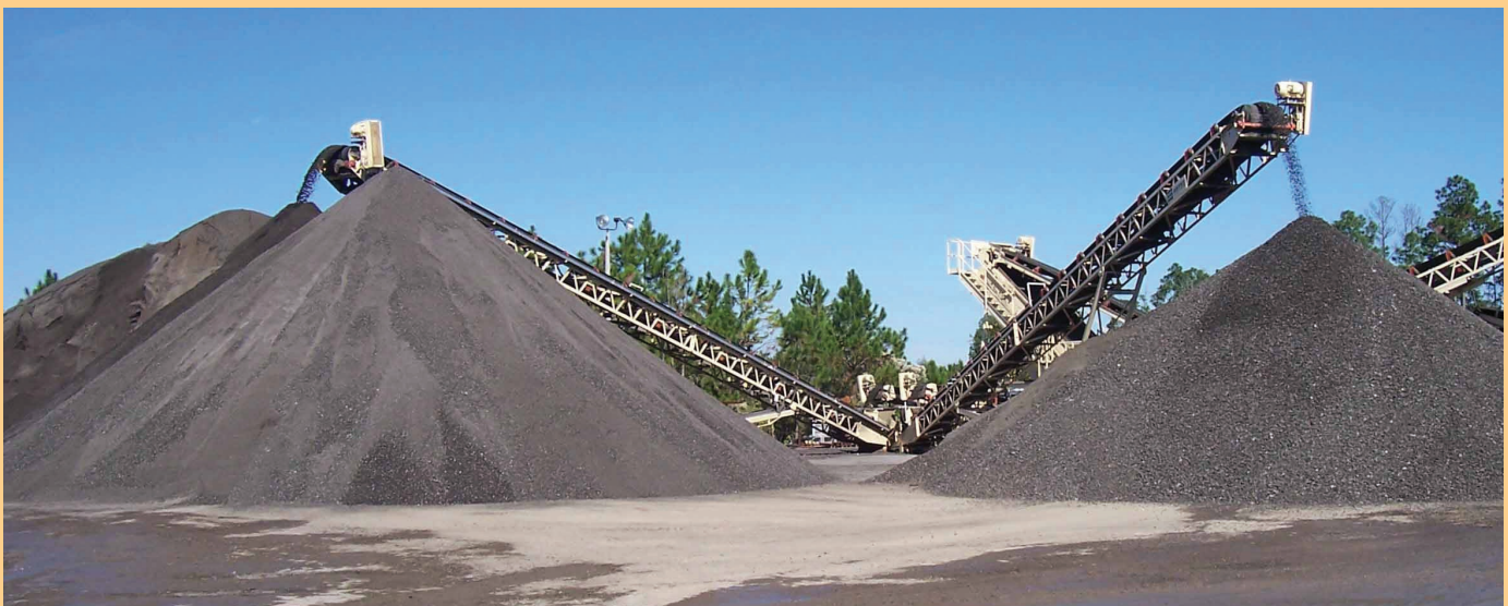
Conveyors deposit piles of fractionated RAP into stockpiles at an HMA supplier in Florida.
