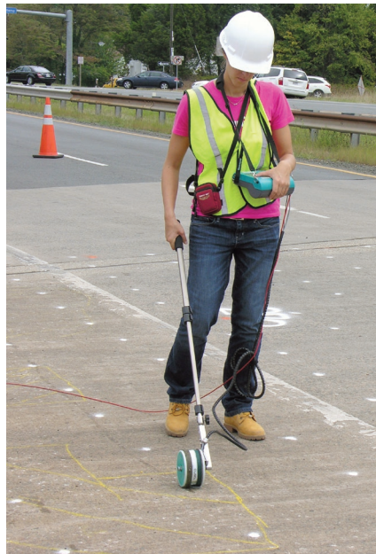
This woman, a researcher at Rutgers University, is conducting half-cell corrosion potential testing on a bridge deck in northern Virginia. Half-cell testing provides information about the likelihood of active corrosion.
