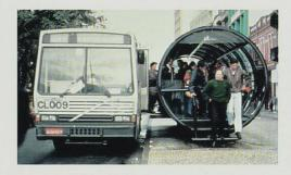
Curitiba's bus system is composed of a hierarchical system that includes a range of services from small feeder minibuses to conventional buses. The backbone of the bus system is composed of express buses operating on five main arteries leading into the city center. This backbone, aptly described as Bus Rapid Transit, is characterized by the following features:
