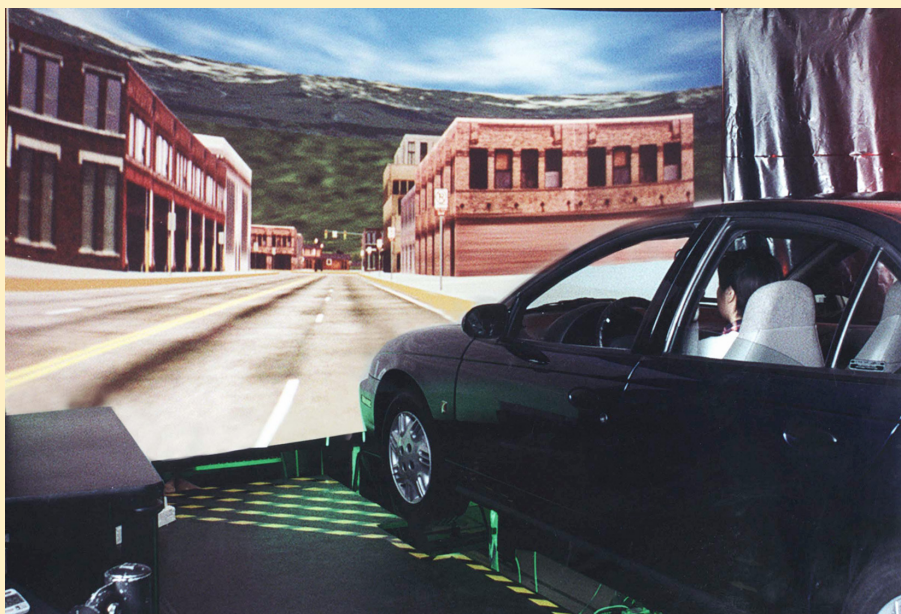
Researchers at TFHRC use the highway driving simulator (shown here) to study nighttime visibility on rural roads and other driving circumstances.
