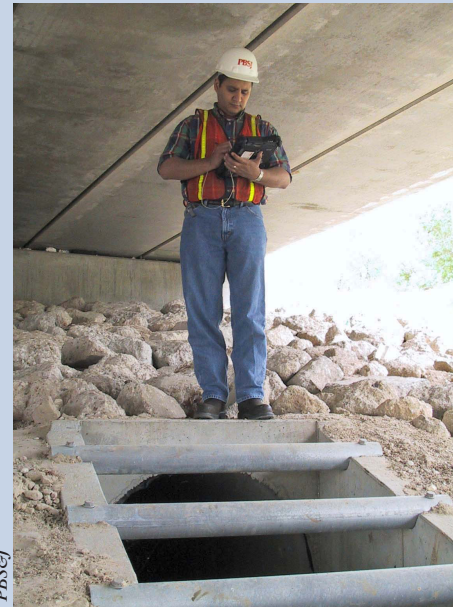
An inspector records information about an outfall located under a highway overpass. In situations such as this where the overpass blocks transmission of GPS satellite signals, inspectors can define the outfall location by clicking on a detailed aerial photograph of the site displayed in ArcPad on the tablet computer screen.
