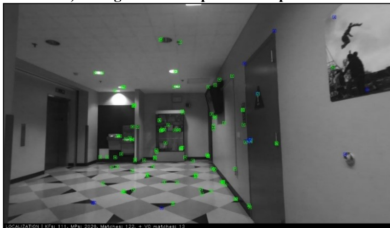
Figure 11: Localization phase of ORBSLAM2 (performed on the third floor of the Engineering building at Cal. State LA). The blue dots represent landmarks.
