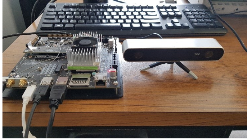
Figure 5: NVIDIA JETSON-TX2 massively parallel GPU and ZED stereo camera used for the implementation of vSLAM.
