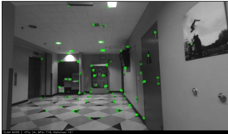
Figure 10: Mapping phase of ORBSLAM2 (performed on the third floor of the Engineering building at Cal. State LA). The green dots represent the points cloud of the environment.
