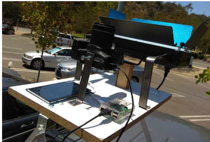
Figure 3: The overall system composed of LED lighting system, DSLR camera, PLUSIII sync system and standalone flash, Raspberry PI, 7" LCD display for programming, and cables.
