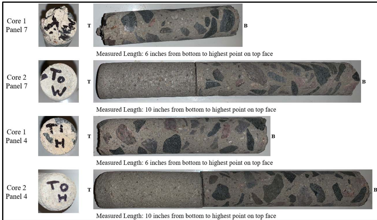
Figure 3-17: Cores and their respective lengths. Lettering “T” indicates the top of the core while “B” indicates the bottom of the core.
