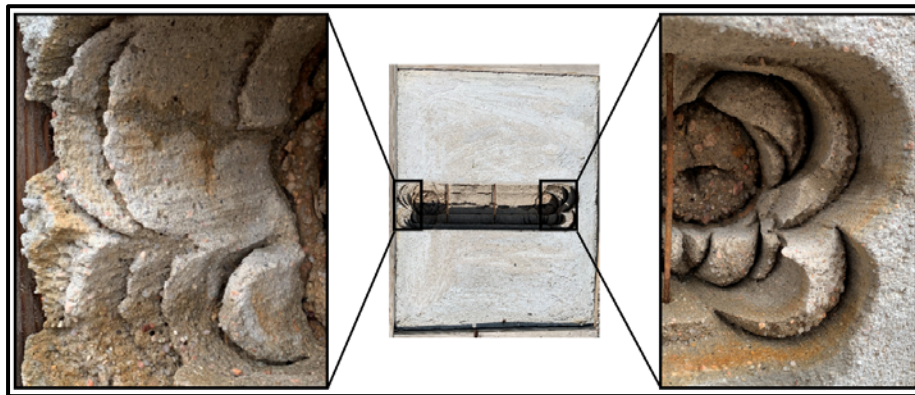
Figure 4-4: Ribs of shotcrete left on edges of panel TEST due to traverse limitations in reversing direction.
