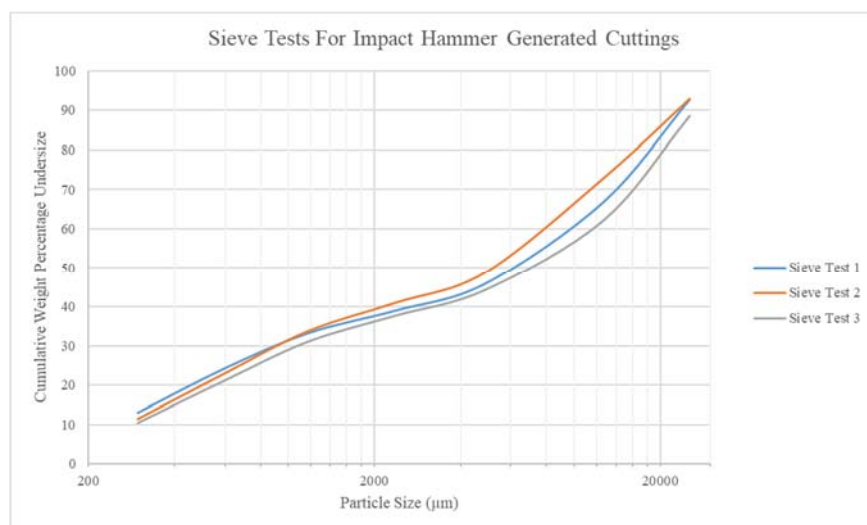
Figure 4-5: Semi-logarithmic plot of impact hammer sieve analysis tests.
