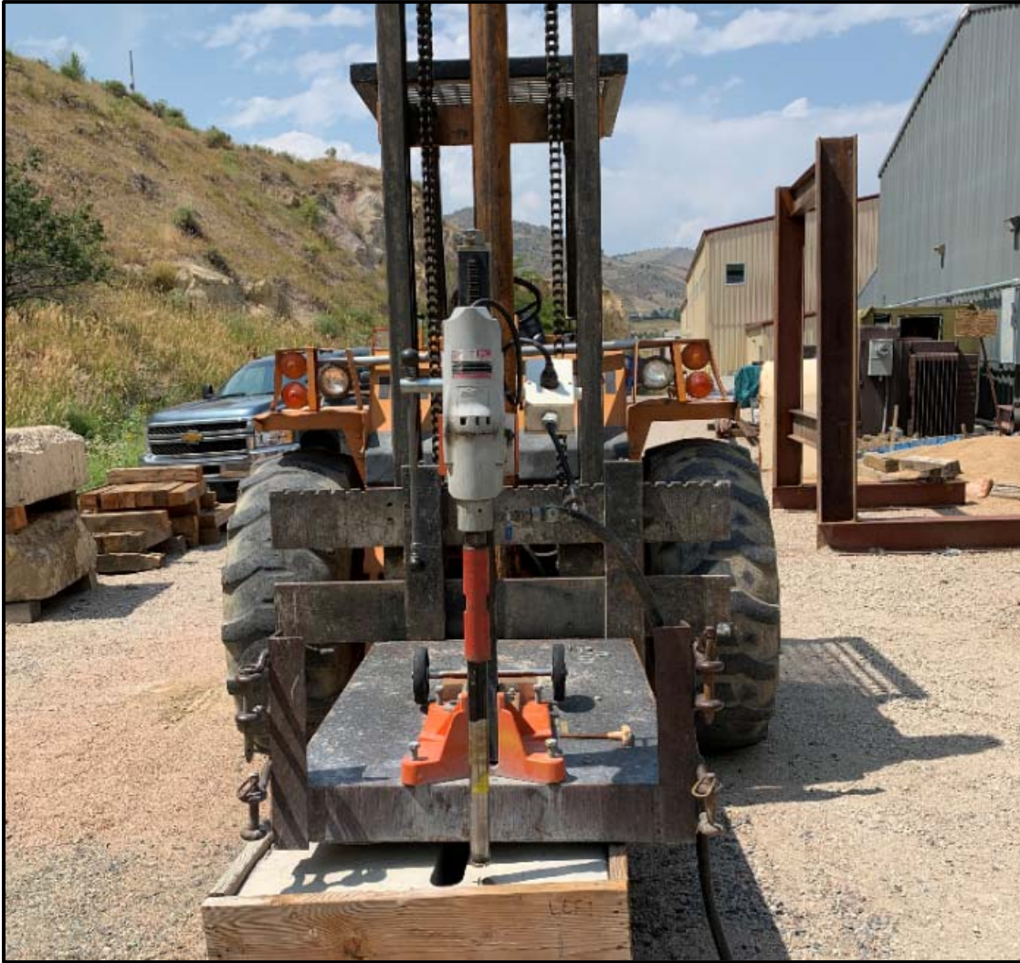
Figure 3-16: Core drill and bit set-up with forklift at EMI.
