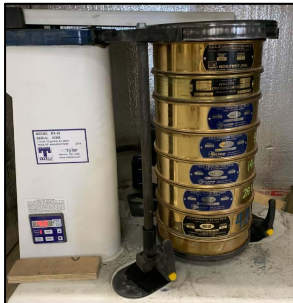
Figure 3-10: Model RX-29 Tyler sieve shaker used for sieve analysis of impact hammer cuttings.
