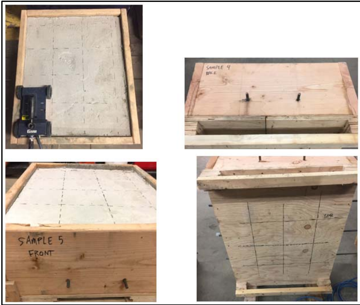
Figure 3-12: Top shotcrete face with GPR gridlines (top left) back timber form face to receive one GPR scan (top right) front timber form face to receive one GPR scan (bottom left) bottom plywood/concrete face with GPR gridlines (bottom right).
