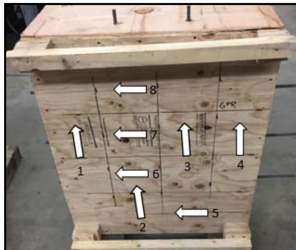
Figure 3-14: GPR scan sequencing for bottom plywood/concrete plan face.
