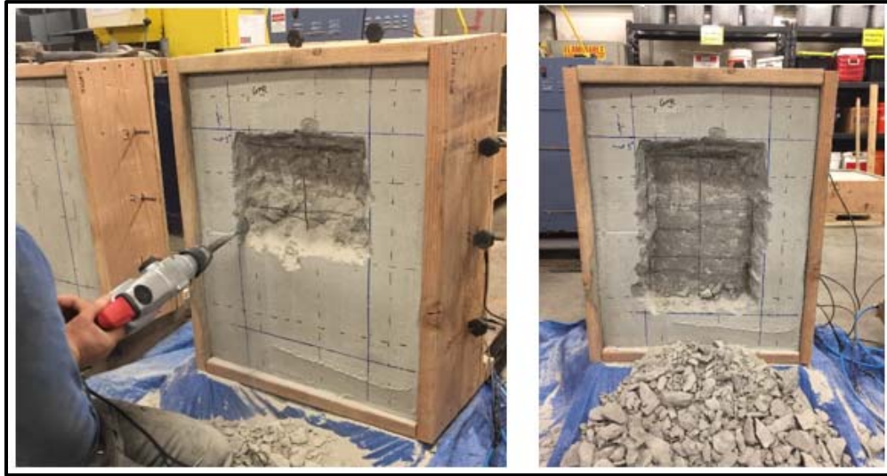
Figure 3-2: Process of mechanical excavation using Bauer impact hammer.
