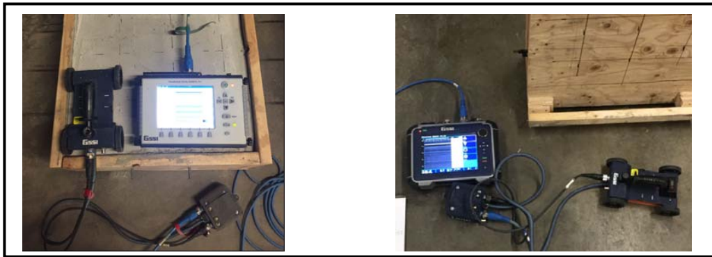
Figure 3-11: 2600 MHz radar antenna connected to SIR 3000 radar system control unit (left) 1600 MHz radar antenna coupled with SIR 4000 radar system control unit.
