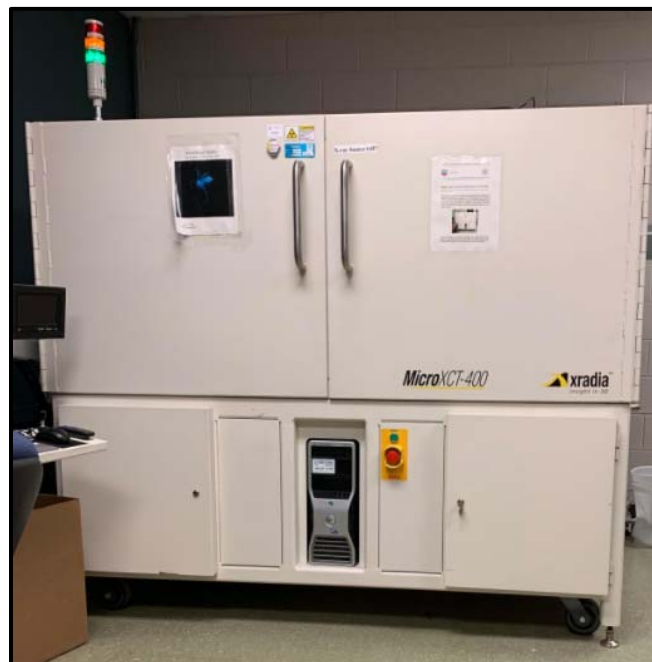
Figure 3-18: MicroXCT-400 equipment used for microCT analysis of core segments.
