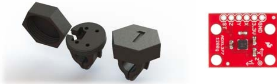
Figure 3-6: Accelerometer mount (left) and ADXL337 (right).
