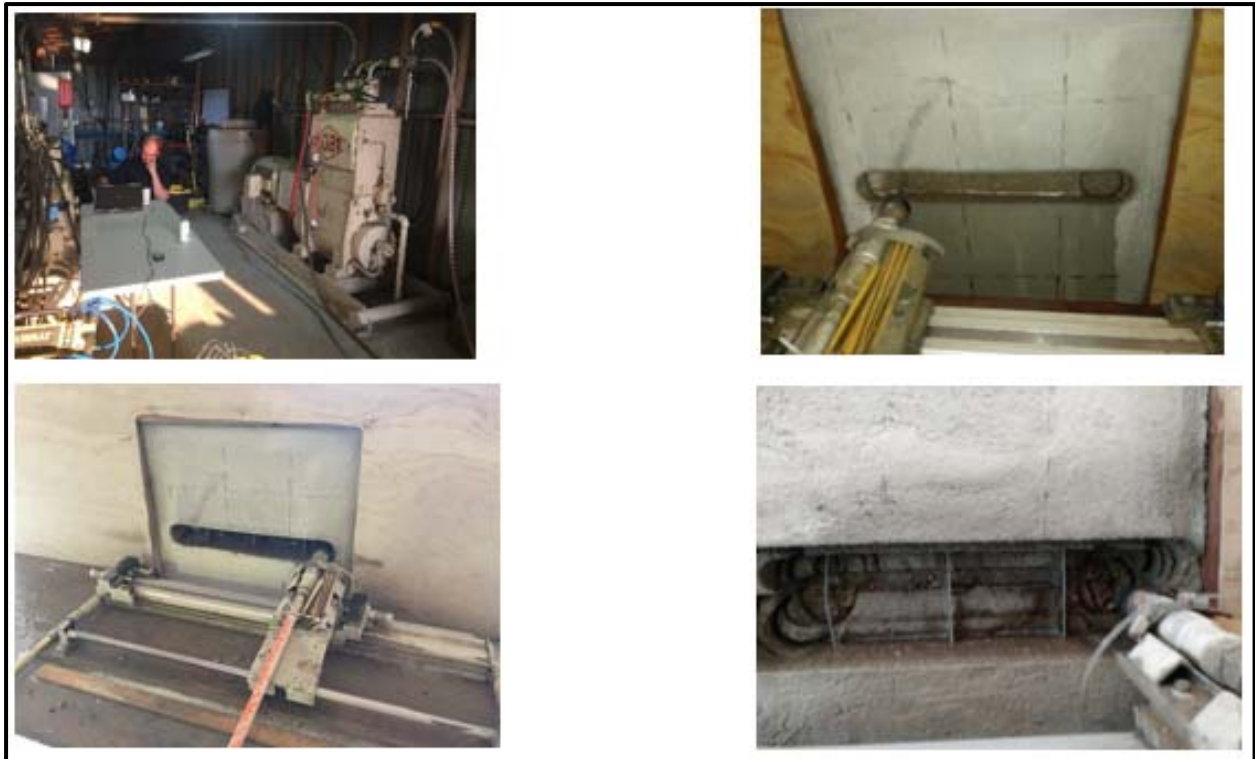
Figure 3-5: Waterjet excavation – SAI/RAMAX Laboratory set-up (upper left) start of slot in panel (upper right) kerf in panel (bottom left) close-up of kerf in panel (bottom right).
