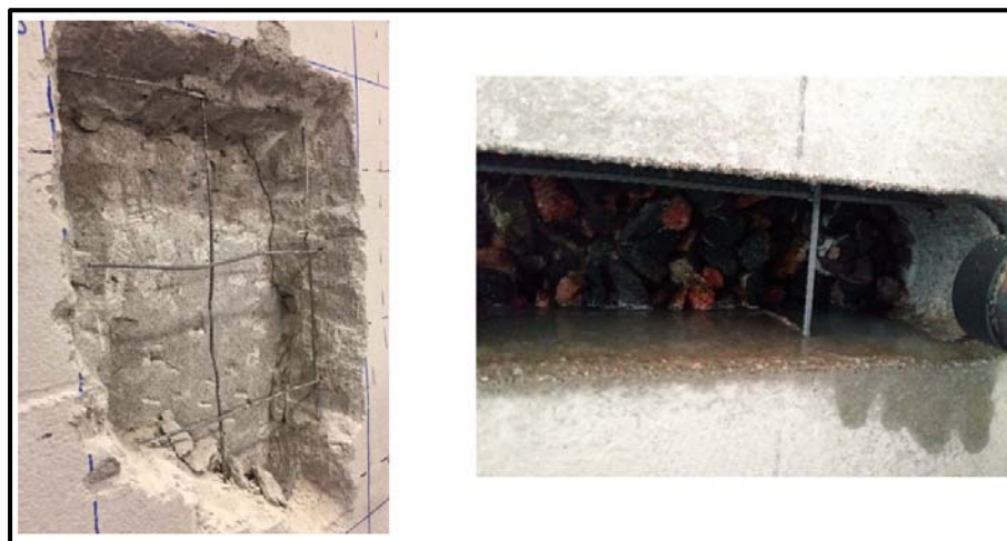
Figure 4-1: Photos taken at panel face showing cutting geometry and bond surface left after impact hammer testing (left) and waterjet testing (right).
