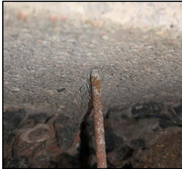
Figure 5-1: Example of edge effect caused by wire mesh, blocking erosion by waterjet, leaving shadow of shotcrete behind steel reinforcement.
